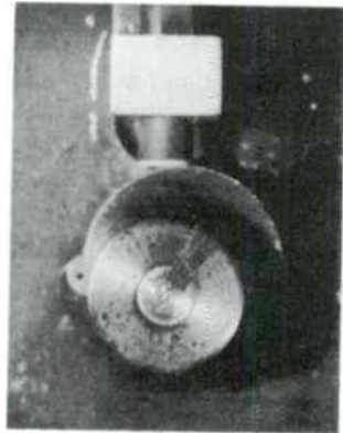
Figure 16-3. Sequence of photographs showing misbehaving cam and follower. The cam is rotating at 2000 rpm. The photographs were taken with stroboscopic illumination at different phases of the cam cycle to show the bouncing action when the cam rotates above a critical speed.
