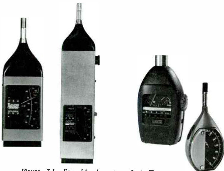
Figure 7-1. Sound-level meters (l.r.) Type 1981-B Precision (ANSI Type S1A), Type 1982 Precision SLM and Analyzer (ANSI Type 1), Type 1565-B (ANSI Type 2), Type 1983 (ANSI Type S2A).
