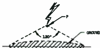
DRAWING 1-A LIGHTNING PROTECTIVE ZONE CREATED BY A SINGLE CONDUCTIVE POINT P, SUITABLY GROUNDED
