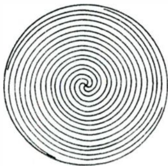
Figure 1-4 PPI Presentation Showing Another Typical Pattern Caused By Interference Between Radars
