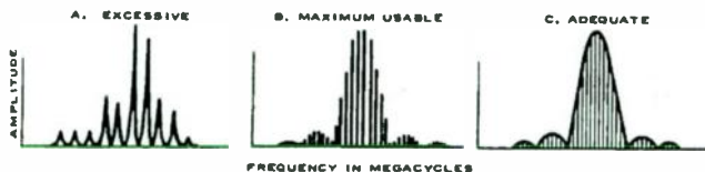
Figure 4-11. Effect of Sweep Frequency on RF Pulse Spectrum
