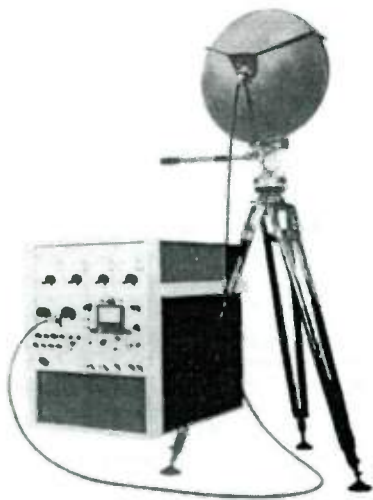
Figure 4-9. Radio Interference Measuring Set AN/URM-138 (Similar to Stoddart Model NM-62A)
