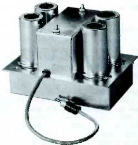
Fig. 4-42. A plug-in stereo multiplex adapter.
