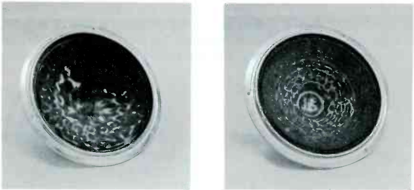
Fig. 6-11. Typical cone breakup at high frequencies.
