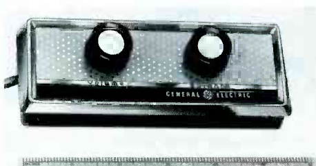
Fig. 5-54. Remote-control unit used with stereo preamplifier to control volume and balance from the listening position.
