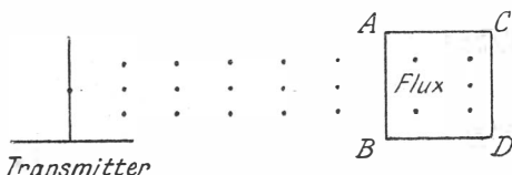
FIG. 139. THE STRONGEST POSITION FOR A FRAME.
