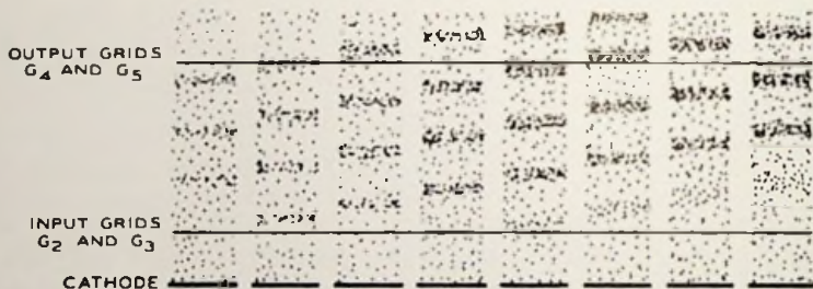
FIG. 7.2. The electron distribution in a klystron indicated at eight different moments. By following the electrons as they progress down the drift tube, the formation of the bunches can be seen.
