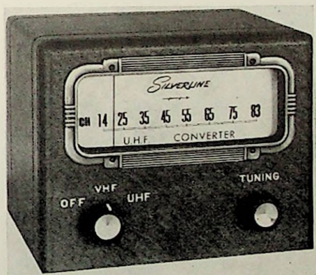
FIG. 12.1. A UHF converter manufactured by the General Instrument Corporation.
