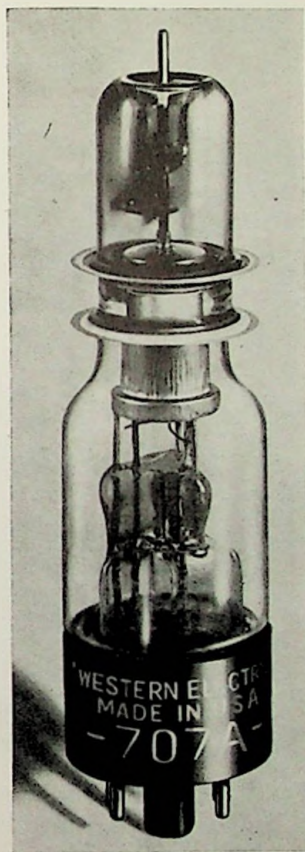
FIG. 7.28. A klystron tube which requires an external cavity resonator. (Courtesy Bell System Technical Journal)
