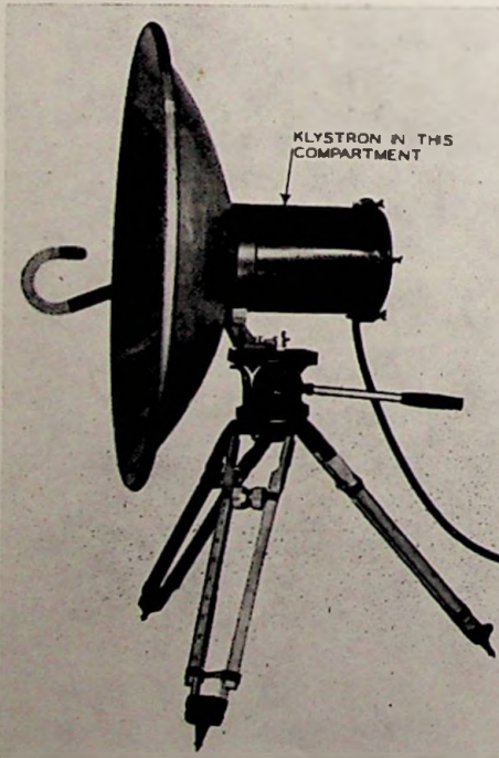
FIG. 7.33A. A klystron reflex oscillator used as the r-f generator in a microwave television relay. (Courtesy RCA)
