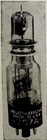
FIG. 1-5.—Type 707A klystron showing disk-seal construction. An external resonator must be connected to the copper disks which extend through the glass envelope. (Courtesy of Bell Telephone Laboratories.)
