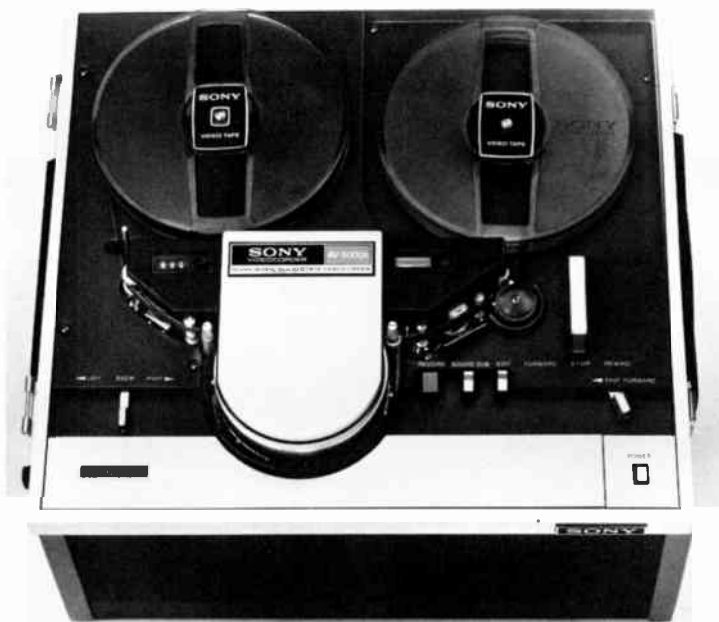
Fig. 8-16 AV 5000A Videocorder. This solid-state helical-scan color recorder uses 1-in. tape and a longitudinal tape speed of 7.5 ips and produces a tape pattern that conforms to the EIAJ Type I VTR Standard. (Sony Corp. of America.)
