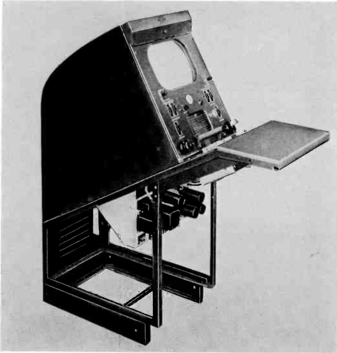
Fig. 4-8. The RCA TS-5A video switcher mounted in a standard console housing with a master monitor. In this arrangement, the fader pushbutton assembly is mounted in the well of the console. (RCA)
