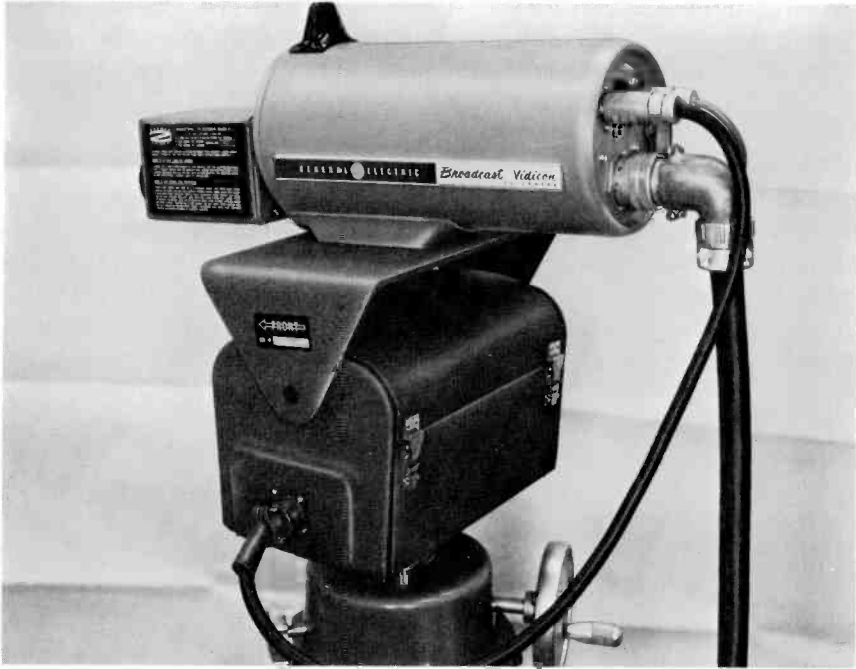
Fig. 4-3. A transistorized studio vidicon camera designed for remote control use, the GE PE-22A. Note that there is no viewfinder. (GE)
