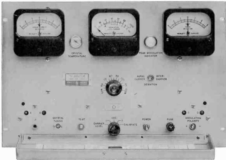
Fig. 5-12. The Hewlett-Packard 335E TV station monitor. (Hewlett-Packard)
