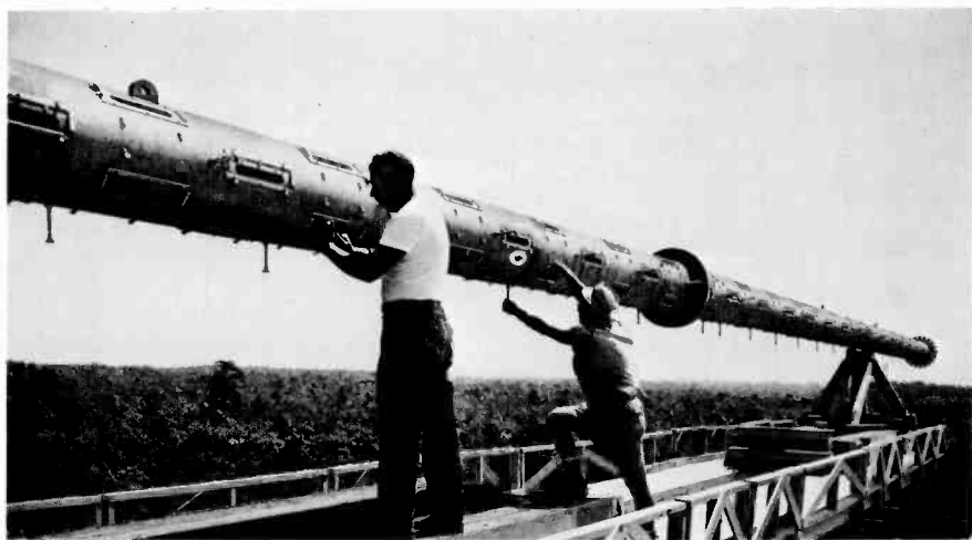
Fig. 7-13. This high-gain uhf pylon antenna is being readied for check-out on the turntable at the factory. The window covers are not yet in place. (RCA)
