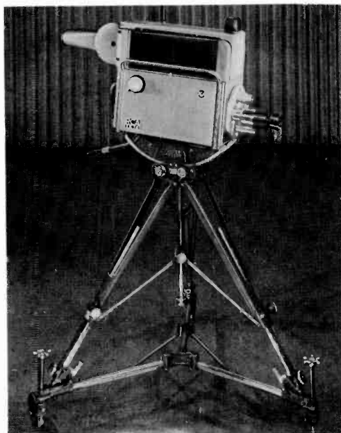
Fig. 3-25. The RCA TK-14, a studio image orthicon camera for monochrome use. This camera, mounted on a portable tripod, uses a 3-inch tube. (RCA)
