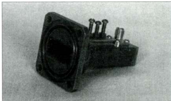
Fig 10.38(b). WG16 to SMA transition (G3PFR). Photo: G6WWM
