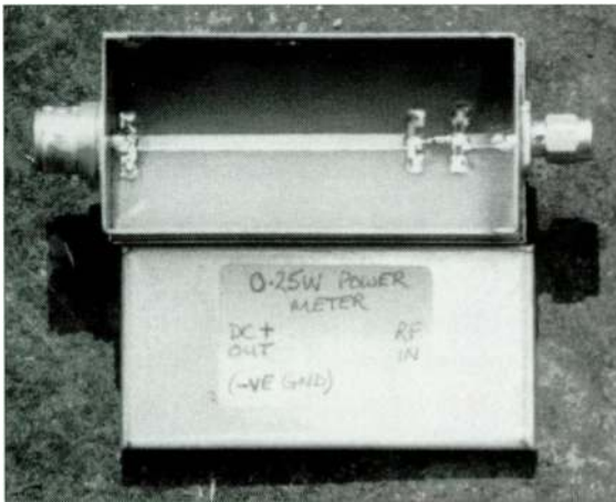
Fig 9.22. (a) Layout of a microstrip and SMD version of the simple milliwatt power meter which will work at 1.3GHz. (b) Photograph of the completed unit (G3PFR)
