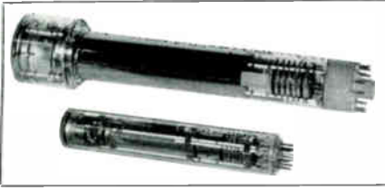
Figure 1.2C. Image Orthicon type pickup tube. Courtesy RCA.
