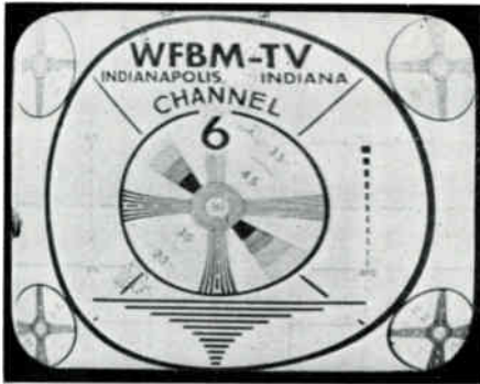
Figure 6.2F. Horizontal sweep non-linearity. Courtesy WFBM-TV.
