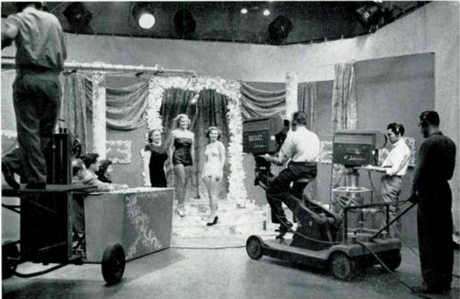
Figure 2.7D. Studio scene at WFIL-TV. The first camera to the right is mounted upon a crane, moved about by the crane operator, shown wearing headphones, at the rear of the dolly. Courtesy RCA.
