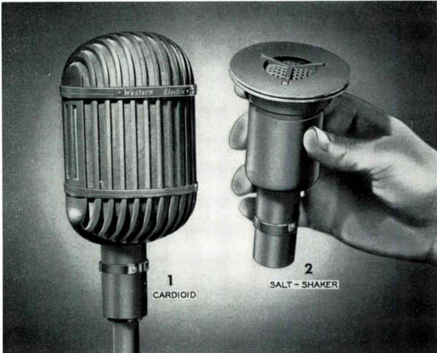
Figure 6.10A. (1) (2) Western Electric Microphones. In (1) is shown the directional (cardioid pattern) mike. In (2) is the non-directional "saltshaker" mike often used in announce booths. Courtesy Western Electric.
