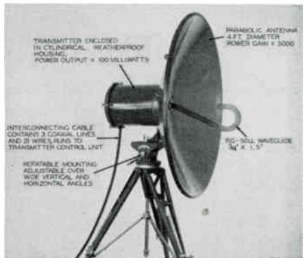
Figure 9.2A. (1) Television Microwave relay transmitter. Courtesy RCA.
