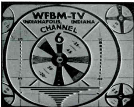
Figure 8.3F. Station test pattern showing effect of reversed polarity smear or transient oscillation. Courtesy WFBM-TV.
