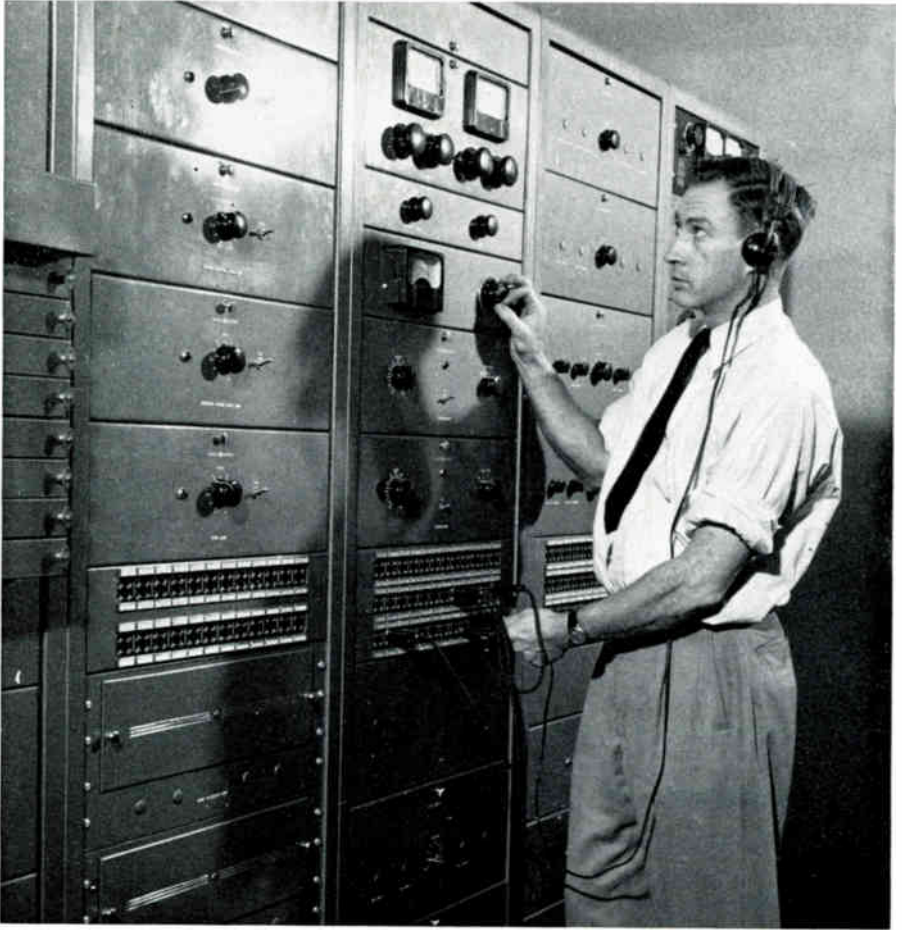
Figure 3.15B. Audio amplifier racks and patch panel in master control room at WRGB. Courtesy General Electric.
