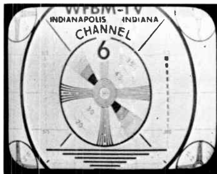
Figure 6.2D. Appearance of test pattern on properly aligned monitor tube when target is underscanned vertically. Courtesy WFBM-TV.
