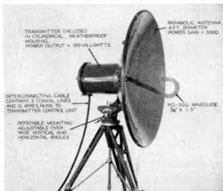
Figure 9.2A. (1) Television Microwave relay transmitter. Courtesy RCA.
