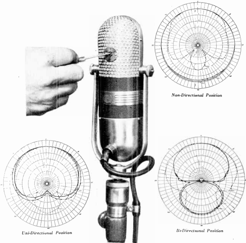
Figure 6.10B. (1) RCA 77-D Microphone showing adjustment of "U," "N," and "B" response patterns.
