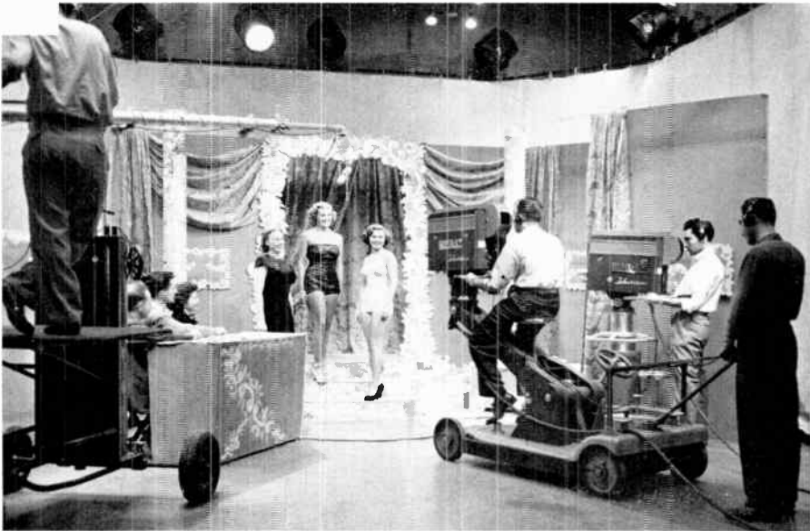
Figure 2.7D. Studio scene of WFII-TV. The first camera to the right is mounted upon a crane, moved about by the crane operator, shown wearing headphones, at the rear of the dolly. Courtesy RCA.
