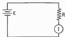
FIG. 27. Ammeters are connected in series with the resistance into which the current flows.
