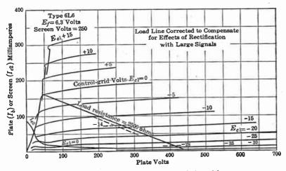
FIG. 19-12. Plate voltage-plate current characteristics of beam-type power tube.
