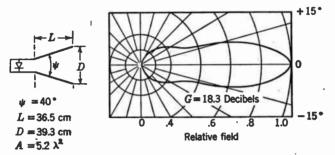
FIG. 15-21. Directional characteristics of a metal horn-type antenna operating on 15.3-cm wavelength. The flared part of the horn is 36.5 cm long; the opening is 39.3 cm.
