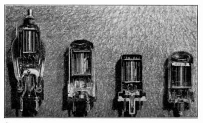
Constructional details of 6J7G. 6SJ7GT, 6SJ7, and 6C7. Courtesy of Sylvania Electric Products Co.
