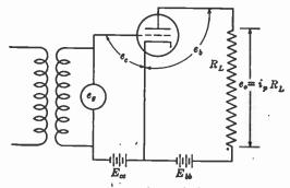
FIG. 3-12. Lower-case letters  $(e_{\theta}, i_{\theta}, \text{ etc.})$  indicate a-c values; capital letters  $(E_{ee}, E_{bb}, \text{ etc.})$  indicate d-c values.
