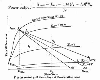
FIG. 20-12. Method of determining correct load resistance for a pentode power tube.
