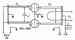
FIG. 7-21. Push-pull 2½-meter, 45-watt oscillator, RCA-1623 tubes;  $C = 15 \ \mu\mu f$ ; R = 1000 ohms, 5 watts;  $L_1$  and  $L_2 = 12$ -inch lengths of ½and ½-inch metal tubing, spaced 1 inch and 1½ inches between centers, respectively; plate voltage = 500 for CW; plate current = 200 ma.
