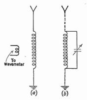
FIG. 6-10. To measure the capacitance of an antenna.
