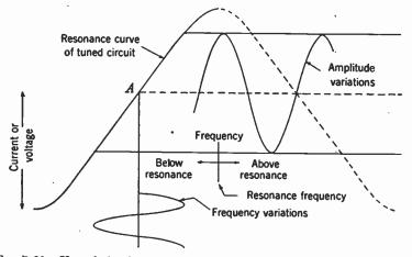
F10. 7-20. Use of simple resonant circuit to convert frequency variations into amplitude variations.
