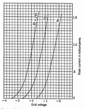
FIG. 5-11. Typical  $E_{\bullet}$ - $I_{\bullet}$  curves. Note that the several curves corresponding to different plate voltages are parallel and have long straight portions.
