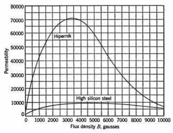
FIG. 11-5. Comparison of two types of magnetic core materials, showing greater permeability of the alloy Hipernik.
