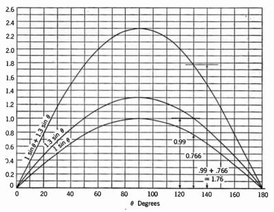
Fig. 10-8. How two sine waves of the same frequency but different amplitudes may be added by means of graph paper.
