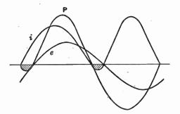
FIG. 27-8. In this case the circuit is slightly capacitive; some power is stored in the capacitor, but most is used up in the resistance of the circuit.
