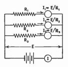
FIG. 11-2. A parallel circuit.
