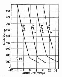
F10. 3-13. Characteristics of shieldgrid thyratron. Note that various starting voltages are possible, depending upon voltage of shield grid.
