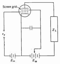
FIG. 13-12. Screen grid has a positive d-c potential with respect to cathode and is by-passed to cathode to provide low-impedance path for alternating currents.
