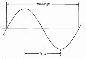
FIG. 6-9. A wavelength is the distance between any two corresponding portions of two waves. Thus, the wavelength may be the distance between two positive (or two negative) peaks, or between the points shown above.
