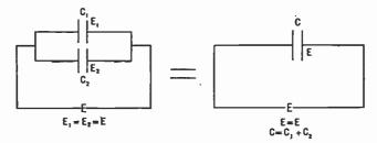
FIG. 4-7. Condensers in parallel.
