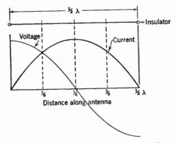
Fig. 5-19. Current and voltage distribution along half-wave antenna.
