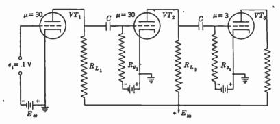
FIG. 4-14. A three-stage amplifier coupled with RC intertube networks.
