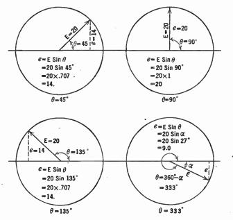
FIG. 5-8. At various times in the cycle the instantaneous value, e, of the vector E is as shown in these vector diagrams.
