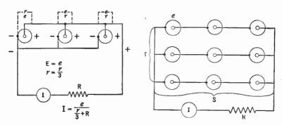
FIG. 5--4. Cells in parallel.
