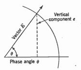
FIG. 6-8. The maximum value of the vector is E; the instantaneous value is  $e = E \sin \theta$ .
