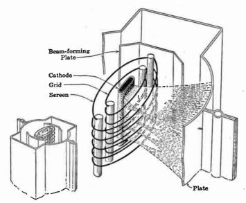
FIG. 18-12. Construction of beam power tube showing beam effect on electron flow.
