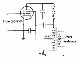
FIG. 12-18. Circuit in which both plate and screen voltages are modulated.
