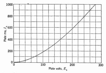
FIG. 3-11. Typical diode plate current curve for a fixed value of filament voltage sufficient to supply all the electrons that will be collected by the plate.
