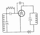
FIG. 3-17. Feedback through grid-plate capacitance.
