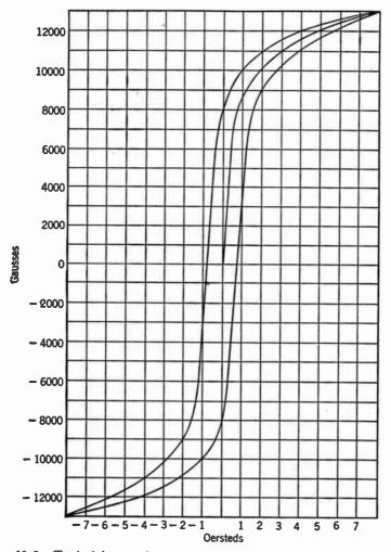
F1G. 10-5. Typical hysteresis curve. Note that as H in oersteds is increased, B in gausses does not increase in proportion but at a slower rate and that as H is decreased, B follows a different curve.
