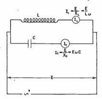
FIG. 8-9. A circuit in which parallel resonance occurs. A parallel circuit like this is sometimes called an antiresonant circuit.
