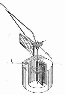
FIG. 4-3. Details of an iron-vane current-measuring instrument.
