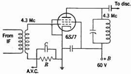
F16. 5-20. Circuit of simple limiter using low plate and screen voltages.
