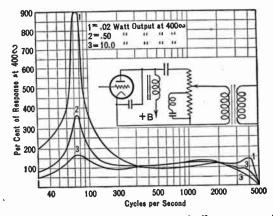
FIG. 20-14. Circuit and response of acoustically compensated volume control.
