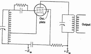
Fig. 10-17. Electron-coupled oscillator.
