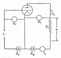
FIG. 1-12. Basic amplifier circuit with resistance load  $R_L$ .
