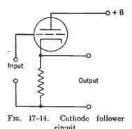
fication in the circuit, which merely serves as a coupling device or transformer between a high-impedance source and a low-impedance load.
