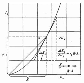
F10. 9-11. Difference between d-c and a-c resistance of a tube. One (a-c) is the slope of the curve; the other (d-c) is merely the ratio between  $I_b$  and  $E_b$ .
