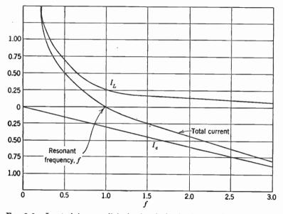
F10. 9-9. In studying parallel circuits, it is simpler to plot the current taken by the reactive branches than to plot the individual reactances as is done in series circuits, for example in Fig. 4-9.
