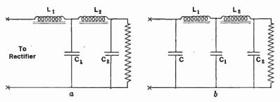
FIG. 12-13. Two types of filter: (a) inductance input; (b) capacity input.
