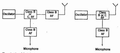
FIG. 7-18. Modulation can take place anywhere between oscillator and antenna. At left is a low-level system; at right, a high-level arrangement.
