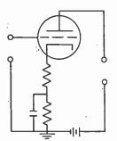
FIG. 15–14. Feedback circuit in which part of the cathode bias resistance is not bypassed. be gained by the use of feedback, for the low plate resistance, 800 ohms, keeps distortion due to loud-speaker-impedance variations to a low value.
