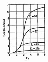
FIG. 2-11. Curves of typical diode, showing that plate current is controlled by plate voltage,  $E_{p}$ , and filament voltage,  $E_{g}$ .
