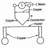
FIG. 2-3. Use of thermoelectric effect as a means of measuring current.
