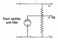
FIG. 17-13. Circuit using voltage regulator tube, such as the 874, to maintain 90 volts across terminals marked.
