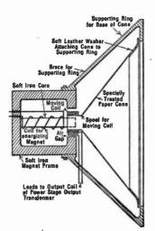
FIG. 14-16. Modern "dynamic" or moving-coil loud speaker.
