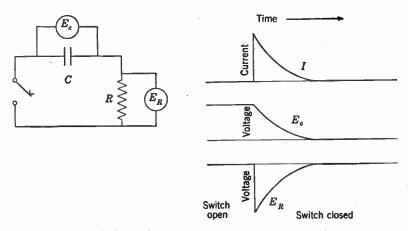
FIG. 16-9. In this figure the condenser is charged. When the key is closed, current flows through the circuit, building up a voltage across R which opposes  $E_c$ . When the charge in C has been dissipated, current ceases and  $E_c$  and  $E_R$  both become zero.
