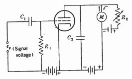
FIG. 4-22. Use of battery and rheostat for bucking out of the plate current meter the steady no-signal current.
