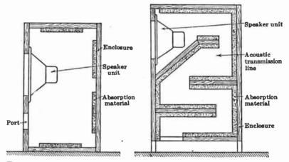
FIG. 18-16. Bass reflex housing for improving low-frequency response of dynamic speaker.
