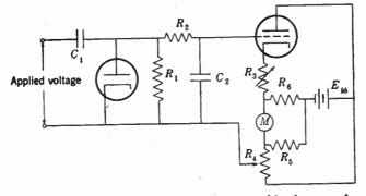
FIG. 7-22. Diode rectifier plus d-c amplifier to enable the use of a more rugged indicating instrument.
