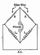
FIG. 7-6. If A and B are so adjusted that there is no sound in the phones,
