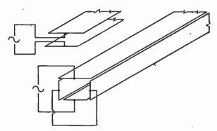
FIG. 8-21. The beginning of a wave guide—two parallel plates. If additional plates are added as in the lower picture, and if all four plates are soldered or welded together (or if a pipe is employed instead) electric energy will flow through the guide without the necessity of a "return" conductor.
