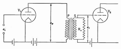
FIG. 10-14. Transformer-coupled amplifier.
