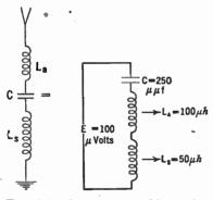
FIG. 19-8. An antenna and its equivalent.
