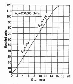
FIG. 13-15. Typical characteristic curve of plate circuit detector.
