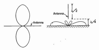
FIG. 8-19. Pattern of radiation from horizontal and vertical doublets located above ground.
