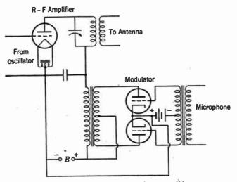
FIG. 11-18. Plate-modulated r-f amplifier.
