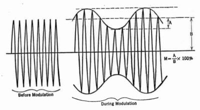
FIG. 2-15. Unmodulated and modulated wave.
