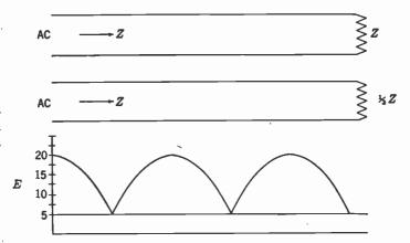
FIG. 5-18. If the line is terminated in a load equal to the line impedance, maximum power will be absorbed by the load. But if the load has a lower or higher impedance, standing waves of current and voltage will occur along the line caused by power flowing back from the load toward the source.
