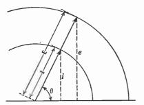
FIG. 12-8. Current and voltage in phase. The maximum value of voltage is greater (or is drawn to different scale) than the maximum value of the current. vectors, which may or may not have the same length, rotating at the same speed.
