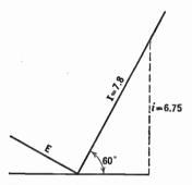
FIG. 14-8. Current lagging behind the voltage by 90 degrees.  $i = I \sin (\theta - 90^{\circ})$ = 7.8 sin (150° - 90°) = 7.8 sin 60° = 7.8 × 0.866 = 6.75 amp
