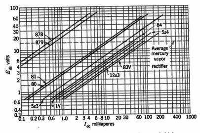
FIG. 1-13. Voltage drop versus current drain of several high-vacuum rectifiers. Note the dotted line at 15 volts representing the drop across a typical mercury-vapor rectifier.
