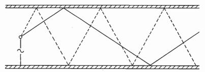
FIG. 9-21. How radiation is reflected by inner walls of a wave guide just as light may be sent down a glass pipe or tube.
