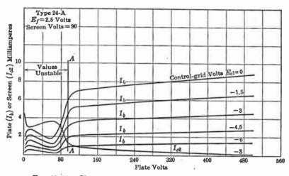
FIG. 12-12. Characteristic curves of typical screen-grid tube.
