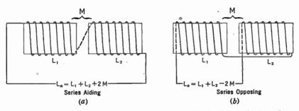
FIG. 5-6. Coils may be connected so that their fields aid or "buck." In one the total inductance is increased; in the other the total inductance is less than either of the component inductances.
