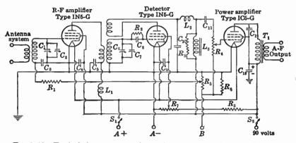
FIG. 3-16. Typical short-wave receiver using one stage of r-f amplification and a regenerative detector.
