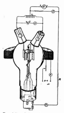
FIG. 2-21. Split-anode magnetron surrounded by electromagnet supplying an external field.
