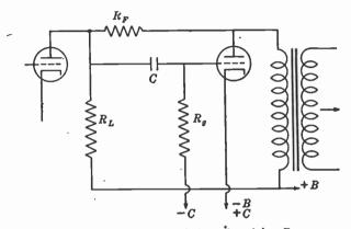
FIG. 16-14. Feedback introduced by  $R_{F}$ .
