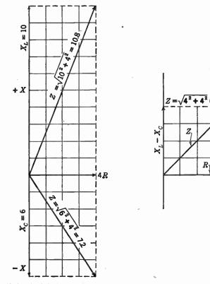
FIG. 18-8. At left is resultant of combining reactances and a resistance to form two Z vectors. At right, the two reactances have been added to form a net reactance of 4 ohms which is then combined with a resistance of 4 ohms to form an impedance of 5.7 ohms.
