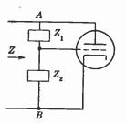
FIG. 2-20. Elements of the reactance tube modulator. Any variation in grid bias changes the phase of Z looking into the points A and B. will be better from the standpoint of noise reduction.
