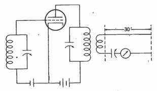
FIG 1-19. Oscillator coupled to a pair of wires to demonstrate concept of radiation resistance.
