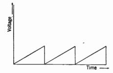
FIG. 8-22. Sawtooth waveform for time base of oscilloscope.
