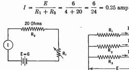
FIG. 10-2. Typical circuit made up of a battery, a rheostat, a tube  $(R_2)$ , and a current meter.
