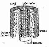
FIG. 15-12. Note how the grid winding has variable pitch from `top to bottom.
