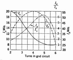
FIG. 7-17. Effect of varying excitation by changing position of center tap in Hartley circuit.
