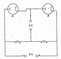
FIG. 7-13. Use of two rectifiers in a voltage-doubling circuit.
