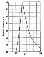
FIG. 2-9. How the antenna current of a radio station varies as the series antenna condenser is varied.
