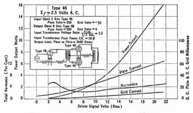
FIG. 12-14. Characteristics of class B amplification.
