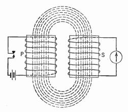
Fig. 1-6. If the coils P and S are coupled so that lines of force from P go through S, a current indicator will show a flow of current in S when the key in P is momentarily closed or open.
