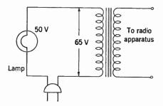
FIG. 16-13. Use of current regulator or ballast tube.
