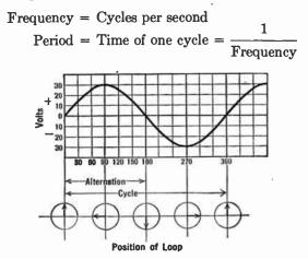
FIG. 14-5. Each position of the conductor as indicated by the arrows corresponds to some voltage as shown on the graph—called a sine wave of voltage.
