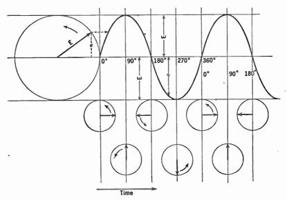
FIG. 1-8. As the vector E rotates, the vertical height, e, of the end of the vector varies according to the curve known as a sine wave. When the vector has the position as shown in the first small circle, the instantaneous value e is zero. At other times the instantaneous voltage has the other values as shown.
