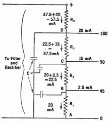
FIG. 14-13. Designing the voltage divider.
