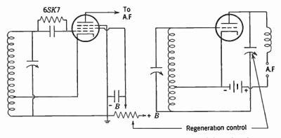
FIG. 4-16. Two feed-back circuits for improving sensitivity of a detector.
