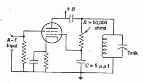
FIG. 3-20. A workable reactance tube modulator which affects the resonant frequency of the tank as though a variable reactance were shunted across the tank.
