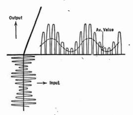
FIG. 4-15. Rectification taking place about a non-linear part of a characteristic.
