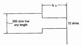
FIG. 14-19. Use of quarter-wave line as a matching transformer between two unequal impedances.
