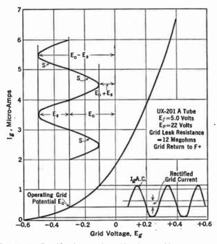
F16. 16-15. Rectification on the grid voltage-grid current curve.
