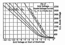
FIG. 2-13. Characteristics of mercury-vapor thyratron. Note that the temperature of the tube affects the starting voltage.
