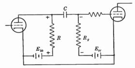
FIG. 1-7. Leakage of current through the condenser C causes a voltage drop across the input of the following tube.
