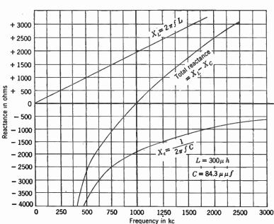
FIG. 4-9. A plot of the reactance of a coil and a condenser in series.  $X_L$  rises in direct proportion to f;  $X_C$  rises inversely as f. The sum,  $X_L - X_C$ , changes from a high negative value where  $X_C$  is greater than  $X_L$ , through zero where  $X_L = X_C$ , to a high positive value where  $X_L$  is greater than  $X_C$ .
