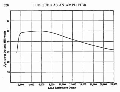
FIG. 6-12. Relation between load resistance, 5000 ohms, and power output. Maximum power is transferred from tube to load when load and tube resistances are equal.
