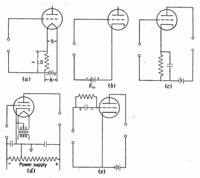
FIG. 15-13. Methods of supplying grid bias.
