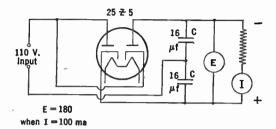
FIG. 8-13. Use of a rectifier with two plates and two cathodes to double the input voltage.
