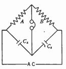
FIG. 16-8. Wheatstone bridge for measuring capacitance. When bridge is balanced, no sound is heard in headphones, and  $C_s = \frac{B}{A}C_s$ .
