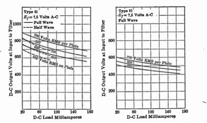
FIG. 13-13. Comparison of condenser-input (*left*) and choke-input (*right*) filter systems. Voltage drops due to resistance of filter chokes are not considered and must be added to these regulation curves if complete regulation data are desired.
