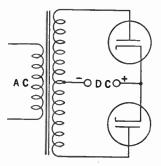
FIG. 6-13. Full-wave rectifier which passes current on both halves of the a-c cycle.
