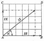
FIG. 21-8. Vector diagram of a series circuit.
