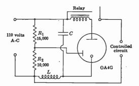
FIG. 4-13. Use of gas tube in a remote-control circuit.
