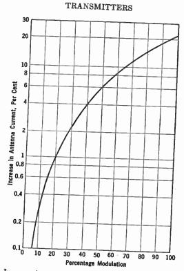
FIG. 13-18. Increase in antenna current as a function of the percentage modulation.
