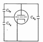
FIG. 6-14. Tube interelectrode capacitances.
