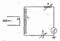
Fig. 1-9. When L is coupled loosely to an oscillator and C is varied, the current indicated at I will go through
