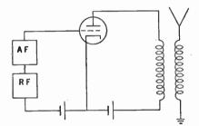
FIG. 1-15. A simple modulating system.
