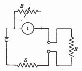
FIG. 9-3. Ammeter-voltmeter method of measuring resistance.
