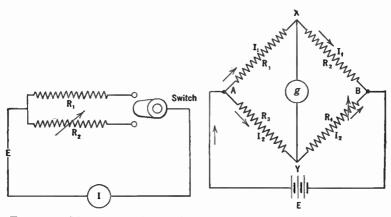
FIG. 11-3. Measuring resistance by FIG. 1 comparison.
