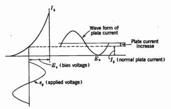
FIG. 1-22. Full-wave square-law vacuum-tube voltmeter.
