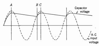
Fig. 10-13. Effect of using an RC circuit with a time constant greater than the time during which the rectifier is not passing current. The condenser maintains part of its charge between cycles of charging current.
