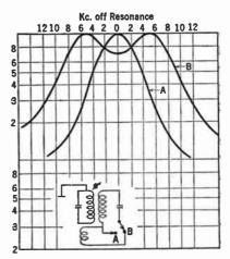
FIG. 11-16. Selectivity curve for twoposition i-f transformer.
