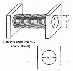
FIG. 2-5. Wire wound on a hollow core to demonstrate that a wire carrying current acts like a magnet.
