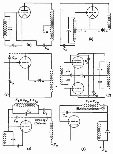
FIG. 5-16. Neutralizing circuits.
