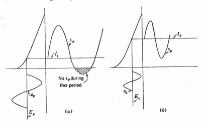
FIG. 5-12. Wrong bias (a) produces an output current and voltage that is not like the input voltage. In (b) the bias is correct.
