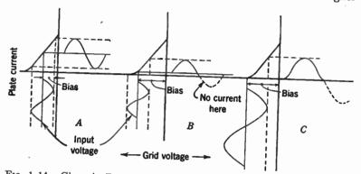
FIG. 1-14. Class A, B, and C amplifiers. Note bias values, portion of characteristic employed, and form of plate current.
