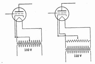
FIG. 21-12. Cathode of heater-type tubes is connected to filament circuit in two ways as shown. This minimizes hum.
