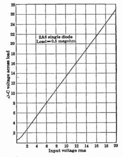
FIG. 9-15. Input-output characteristics of a diode detector.
