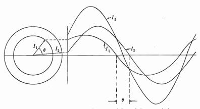
FIG. 8-8. In this curve  $I_3$  is the sum of  $I_1$  and  $I_2$  at each instant.
