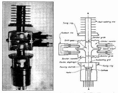
FIG. 16-21. Cutaway and sectional views of the 410-R/2K30 Klystron of Sperry, a tube of the velocity-modulation type which makes possible generation, amplification, and conversion of frequencies in the centimeter wavelength region. The tube is 6 inches long overall.
