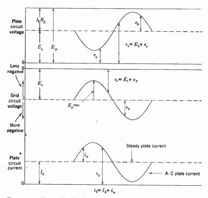
FIG. 10-12. Phase of grid, plate, and load voltage. As  $e_p$  becomes more negative  $e_p$  becomes less negative. The load voltage,  $e_L$ , also differs from the grid voltage by 180 degrees.
