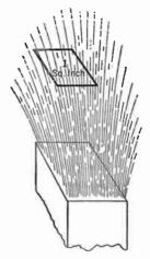
FIG. 3-5. The number of lines of force going through 1 sq in. or other unit of area is known as the flux density.
