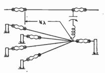
FIG. 7-19. Hertz antenna erected over a counterpoise or artificial ground of low loss.
