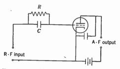
FIG. 15-15. Grid-leak and condenser detector.
