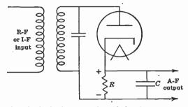
F10. 8-15. Simple diode detector. Rectified voltages appear across R.
