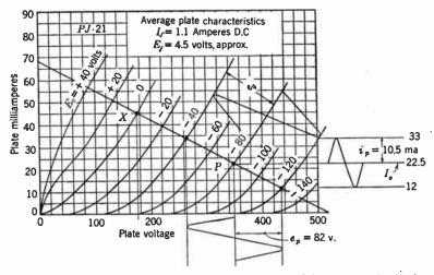
FIG. 7-12. The straight line between  $I_b = 69$  ma and  $E_b = 552$  volts is the "load line." The value of  $I_b$  for any combination of  $E_b$  and  $E_c$  for a load resistance of 8000 ohms may be found from it. The slope of the line  $E_b \div I_b = 8000$  ohms.
