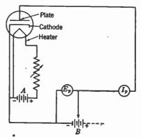
Fig. 1-11. Connections for studying action in a two-element or diode tube. Here the two elements are the cathode and the plate, the heater serving only to heat the cathode to emitting temperature.
