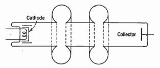
FIG. 13-21. Elements of the Klystron. The circular devices along the tube are cavity resonators.
