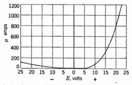
FIG. 7-15. Crystal (Carborundum) detector characteristic.
