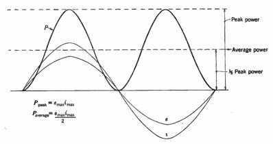
FIG. 7-8. Power is the product of e and i, and the curve marked P is actually secured by multiplying together these factors. Note that the power curve has twice the frequency of the e and i curves.
