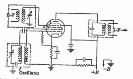
Fig. 7-16. Pentagrid converter circuit for frequency changing.
