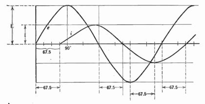
FIG. 13-8. Current and voltage in an inductive circuit where the current lags behind the voltage.
