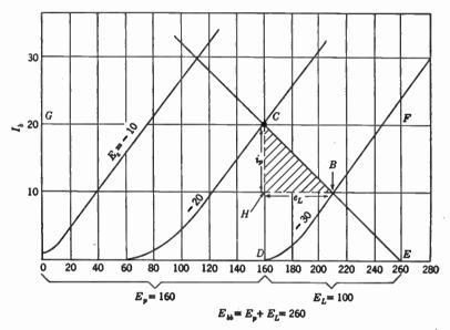
FIG. 8-12. Power diagram for an amplifier with resistance load of 5000 ohms.
