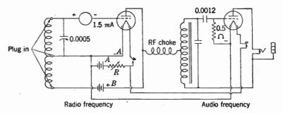
FIG. 4-10. Circuit diagram of a modulated oscillator useful as a wavemeter. The r-f oscillator has a d-c meter in its grid circuit and employs a series of plug-in coils. The modulating oscillator may use an audio output transformer or other center-tapped inductance of the correct value. When the r-f oscillator is coupled to an external tuned circuit, a sharp dip in the grid current will occur when the two circuits are tuned to the same frequency.
