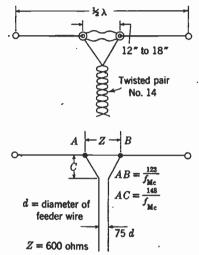
FIG. 12-19. Manner of connecting transmission lines to antenna to produce proper impedance match.
