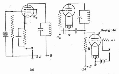
FIG. 6-18. Methods of keying an oscillator or an amplifier. At (a) the plate current is keyed directly; at (b) a keying tube is employed. Voltages across the key in (b) are much lower than in (a).
