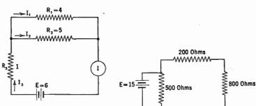
FIG. 12-2. A problem involving both series and parallel resistances.
