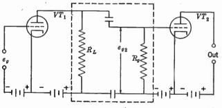
FIG. 2-14. A two-stage resistance-capacitance coupled amplifier.
