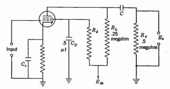
FIG. 8-14. Typical resistance-coupled amplifier using a pentode tube.
