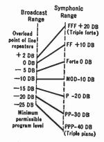
FIG. 21-14. Compression of dynamic range in broadcasting system.
