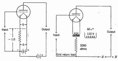
FIG. 22-12. Methods of biasing the grid negative.
