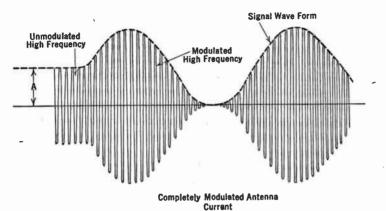
FIG. 10-18. A r-f wave before and after complete modulation.
