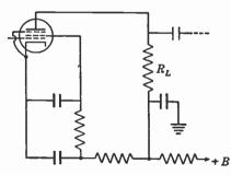
FIG. 18-14. Use of series resistance and shunt capacitance to keep alternating current out of a power supply. See also Fig. 9-14.
