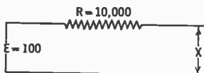
FIG. 7-3. A low-resistance voltmeter placed at X will not read the open-circuit voltage.
