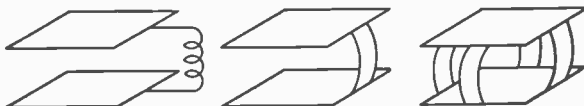
FIG. 12-21. How a cavity resonator may be built up by completely closing in the sides of a two-plate condenser.
