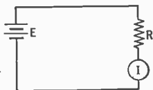
FIG. 5-3. Ammeters are connected in series with the resistance into which the current flows.
