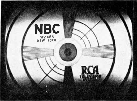
FIG. 230.—60-c.p.s. hum in the video signal circuit.
