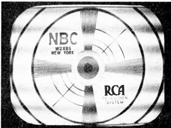
FIG. 235.—Interference from audio frequencies in the signal circuit. May arise from cross-talk anywhere in transmission or reception system, but usually from inadequate trapping of sound intermediate frequencies at 8.25 or 14.25 Mc.
