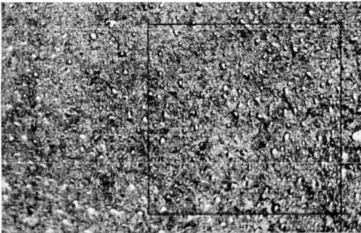
FIG. 49B.—Surface of the iconoscope mosaic, magnified 250 diameters. The square (0.008 inch on a side) is roughly the size of a single picture element.
