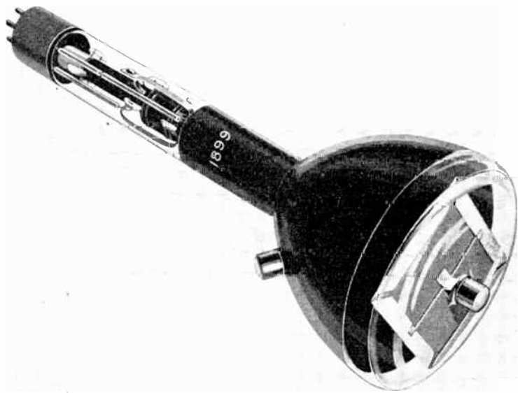
FIG. 301A.—Type 1899 monoscope, a static-image signal generator tube widely used for image testing.
