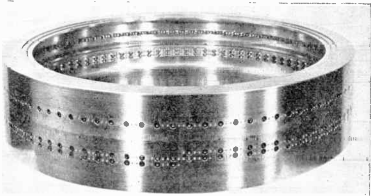
FIG. 46A.—Typical high-speed mechanical scanning drum. The scanning apertures are fitted with lenses to improve the optical efficiency.
