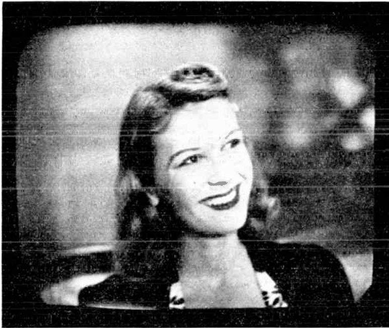
FIG. 56.—Appearance of television image when subject is adequately illuminated and when shading-correction signal has been added to remove effects of spurious shading signal. (Figs. 54, 55, and 56 from Lohr, "Television Broadcasting.")
