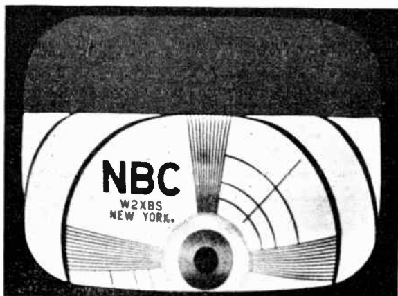
FIG. 238B.—Incorrect positioning due to excessive d-e component in vertical scanning circuit.
