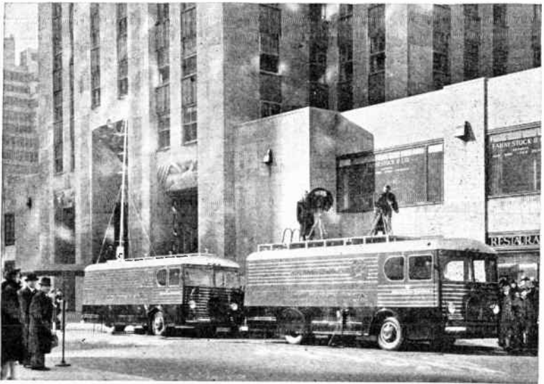
FIG. 275.—Mobile transmitting equipment of the National Broadcasting Company. The pickup equipment (cameras, microphone, and video signal circuits) is in the forward bus, the relay transmitter in the bus at the rear.
