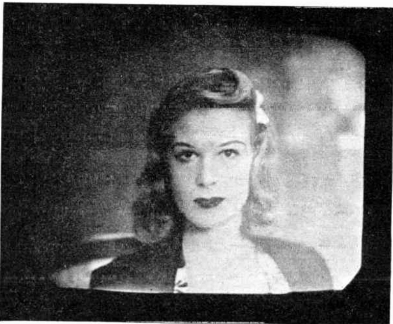
FIG. 54.—Television image showing improper background shading due to the spurious signal generated by redistribution of secondary electrons in the iconoscope. To avoid this defect, a compensating signal must be added (see Fig. 256, page 414).
