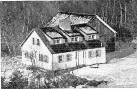
FIG. 2A.—A simple still picture reproduced in a 120-line half-tone engraving. The picture elements (half-tone dots) cannot be discerned except on close inspection.
