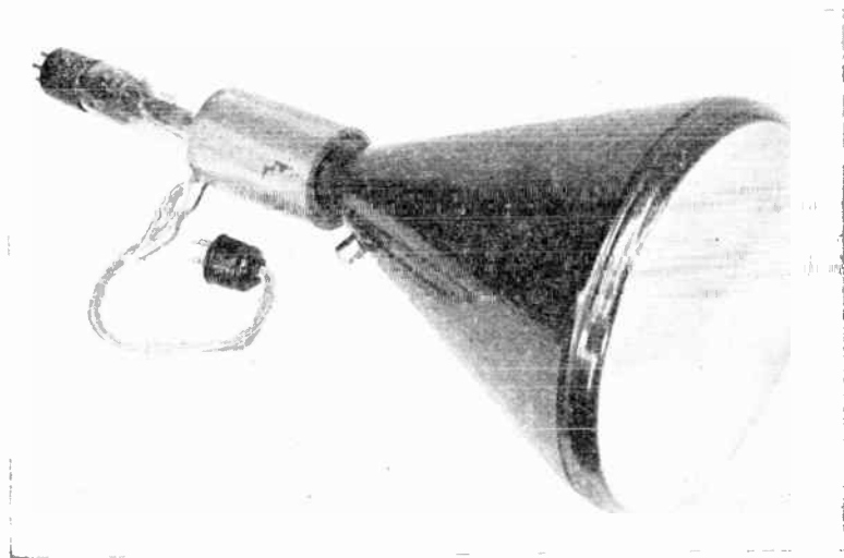
FIG. 85.—Typical magnetically-deflected picture tube. The scanning yoke (cylindrical structure) contains two sets of coils which produce horizontal and vertical deflecting fields at right angles to the axis of the tube.
