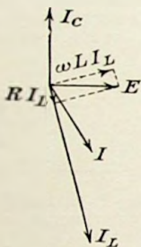
FIG. 69.—VECTOR DIAGRAM OF PARALLEL CIRCUIT.
