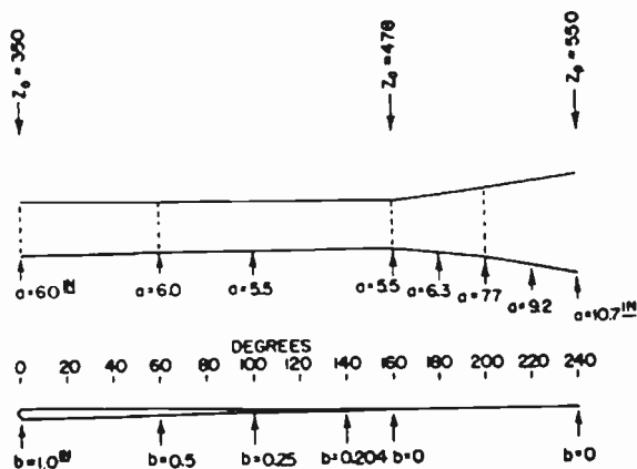
FIG. 4.43. Construction of exponentially tapered matching section from 550 to 350 ohms.
