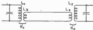
FIG. 28. Link-coupled tuned circuits. Maximum effective coupling is realized when the two links have the same inductance.
