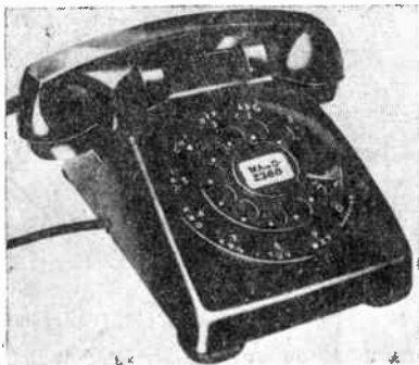
FIG. 3. Typical dial telephone set, 500 type.
