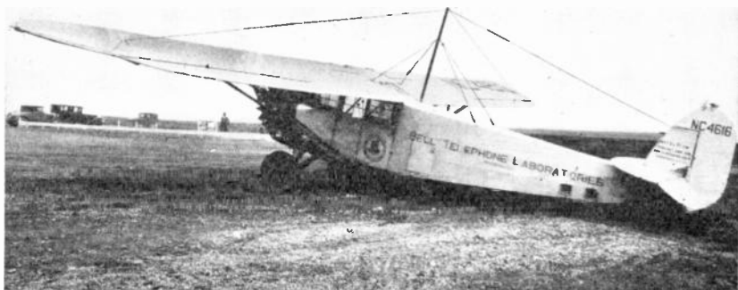
FIG. 312.—Airplane equipped with antenna such as used in short-wave communication between plane and ground.
