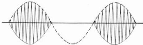
FIG. 221.—Interrupted continuous waves generated by applying an alternating-current voltage directly to the plate of an oscillator.
