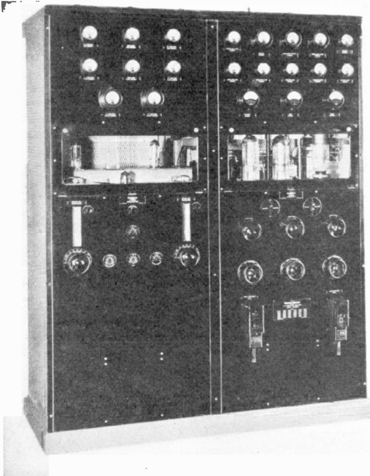
FIG. 231a.—Western Electric 1-kw broadcast transmitter—front view.
