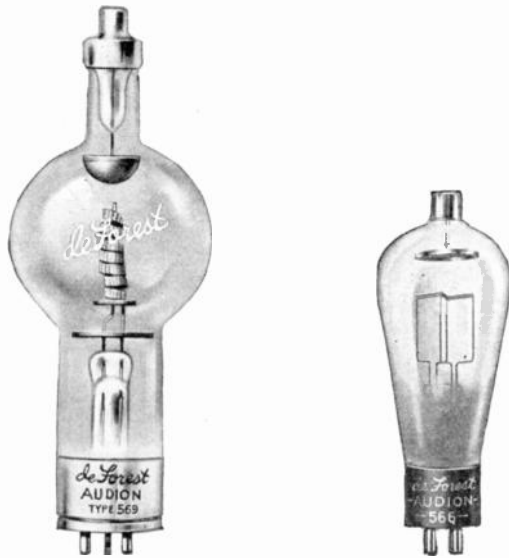
FIG. 208.—Typical hot-cathode mercury-vapor rectifier tubes. Note the small plate, the ribbon-like cathode, and the comparatively large spacing between plate and cathode.
