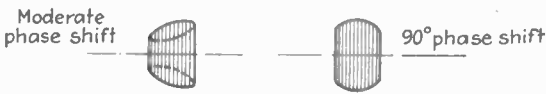
(c) Distortionless modulation with phase shift between modulating voltage applied to the cathode-ray tube and the modulation envelope
