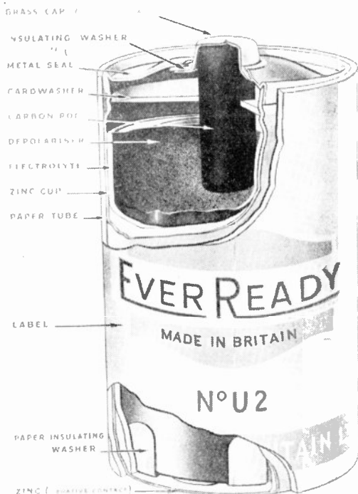
PLATE X.—A Unit-type Dry Cell, Suitable for Supplying up to 0.3 A
