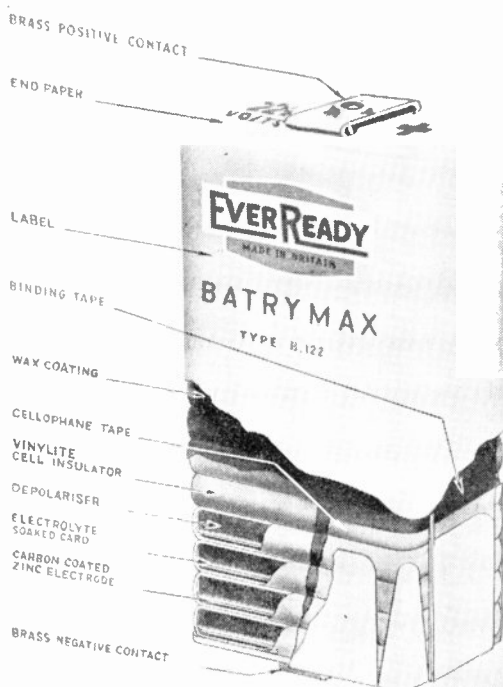
PLATE XI.—A Dry Battery of Layer-type Cells Suitable for miniature equipment; current drain 1 mA.
