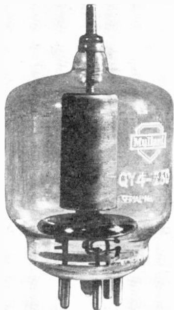
FIG. II.5.—Mullard QY4-250A Tetrode Anode dissipation, up to 250 W; H.T. supply, up to 4 kV; note screen over grid leads.
