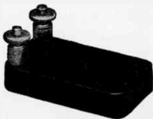
FIG. 23. Fixed receiving condenser.
