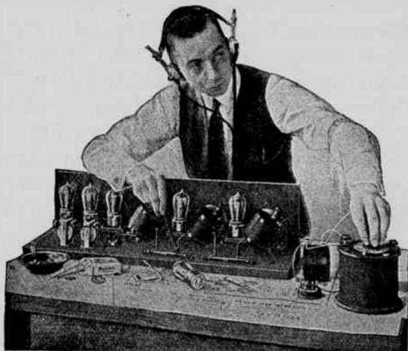
FIG. 97. Showing the five-tube "neutrodyne" receiver being adjusted for complete neutralization.
