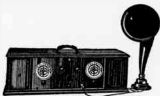
FIG. 51. Modern Super-Heterodyne receiver showing two control handles.
