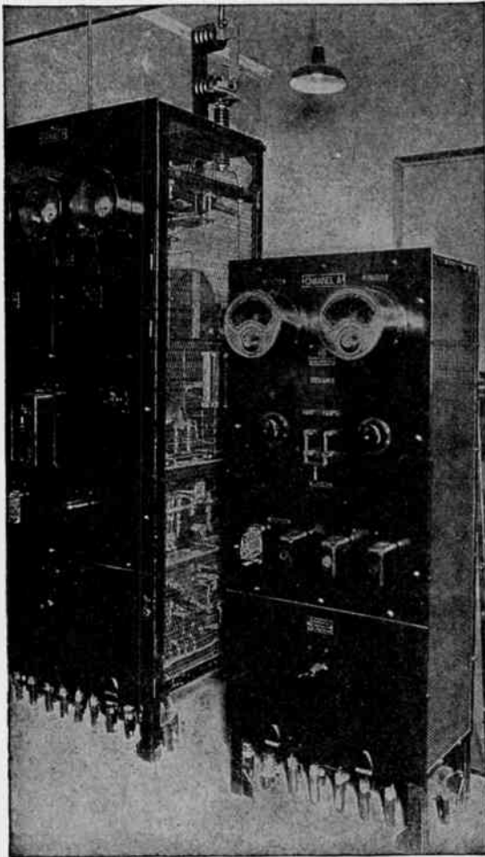
FIG. 71. Radio telephone transmitter unit, high power. Vacuum tube panel (left). Control panel (right).
