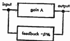
Fig. 3—In negative-feedback amplifier considerations \beta , expressed as a percentage, has a negative value. A line across the \beta and A scales intersects the center scale to indicate change in gain. It also indicates the amount, in decibels, the input must be increased to maintain original output.
