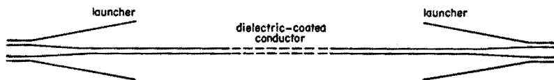
Fig. 17—Surface-wave transmission line with launchers at each end. These form transitions to coaxial line.
