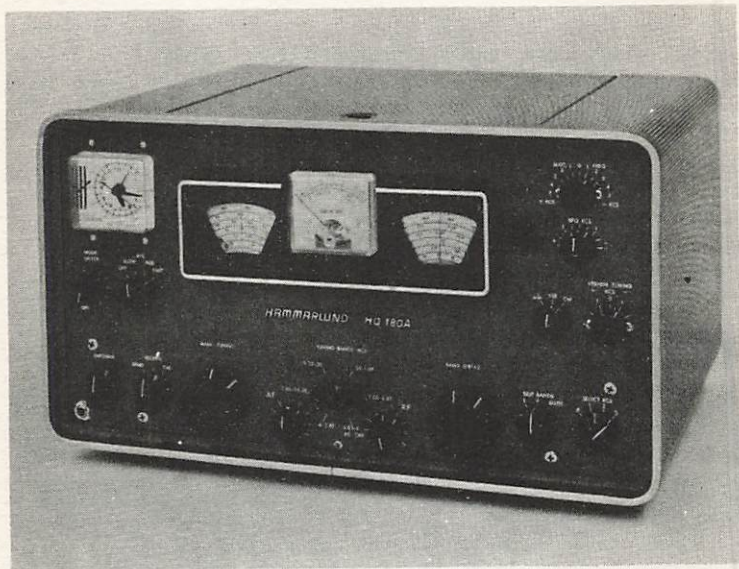
Fig. 6-4. The Hammarlund HQ-180A, a deluxe receiver suitable for the SW listener as well as hams, contains a built-in 24-hour clock.
