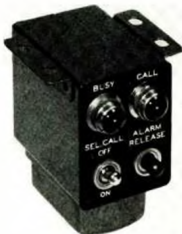
Fig. 8. This dashboard unit carries the decoder controls and the call buzzer
