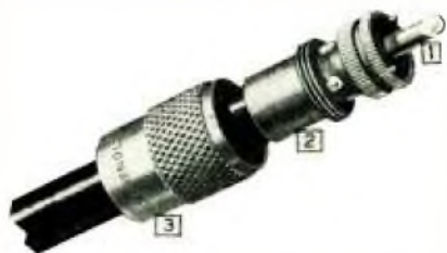
Fig. 32. Be sure that the coupling ring 3 is in place on the cable before the connector shell is soldered to the cable
