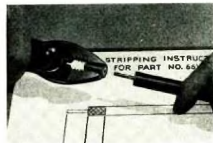
Fig. 34. Remove the insulation and shield
