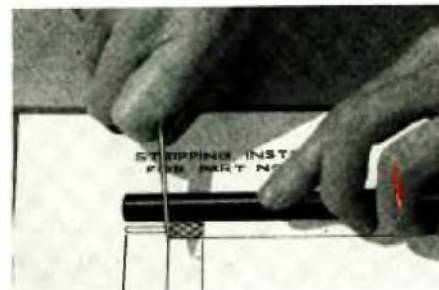
Fig. 33. Cut through to the center wire
