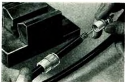
Fig. 37. Slip the shell on to the cable
