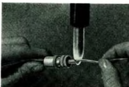
Fig. 40. Solder pin to the center wire
