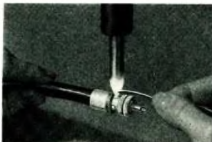
Fig. 39. Solder shell to the cable shield
