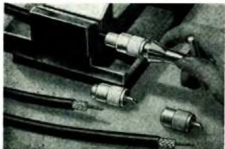
Fig. 38. Screw the shell, as Fig. 31 shows
