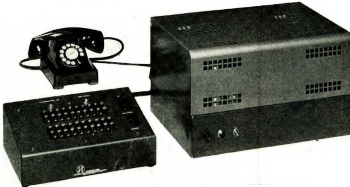
Fig. 2. The push-button selector and coding unit make up the complete selective calling equipment. Telephone indicates size
