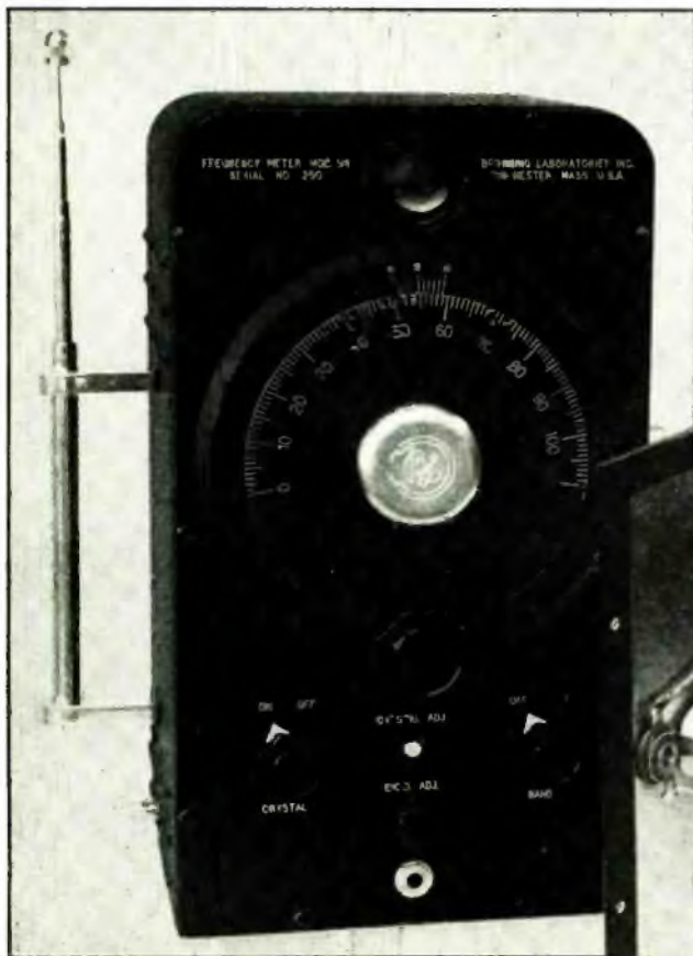
Fig. 20. Browning frequency meter, type S4. Accurate to .002%, it exceeds requirements of FCC.
