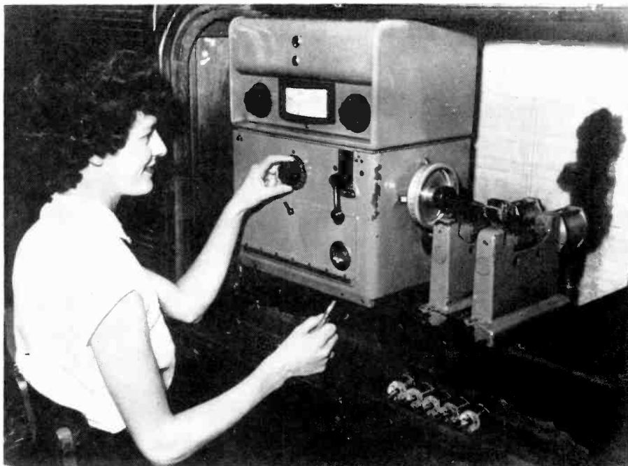
Armature-balancing device used by Garrard of England to check armatures dynamically
