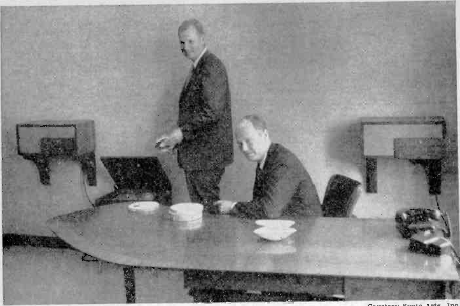
Two infinite-baffle enclosures of the air-suspension type are seen in use in a stereophonic set-up for a business office
