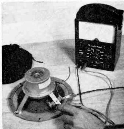
Left: Pictorial and schematic diagrams of a fuse in the speaker line. Below: A simple ohmmeter resistance-checks voice coil
