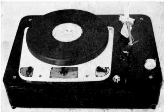
The completed turntable and tone arm assembly rests on a vibrationproof shock-mounted base
