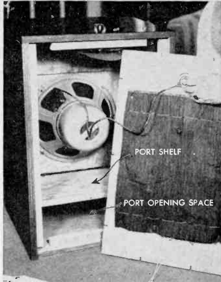
Equipment for evaluation furnished by Allied Radio Corp. Above: The port and the shelf are acoustically important parts of this bass reflex enclosure. Left: A baffle and its folded-side equivalent
