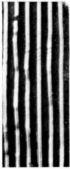
Left: a linear representation of sound in terms of air pressure and distance from the source. Right: 78-RPM phonograph record grooves
