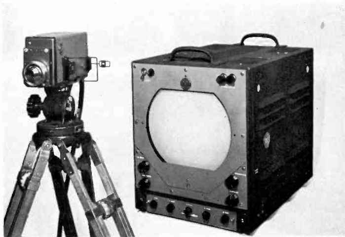
(Above) Miniature camera and compact control monitor — standard equipment for industrial television.
