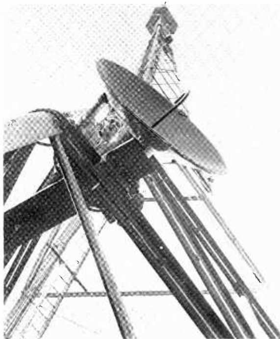
(Above) This RCA microwave relay receiver is used at the studio or transmitter for the reception of TV signals from a mobile unit. (Right) A microwave receiver mounted on the transmitter tower of Station WCAU-TV in Philadelphia.
