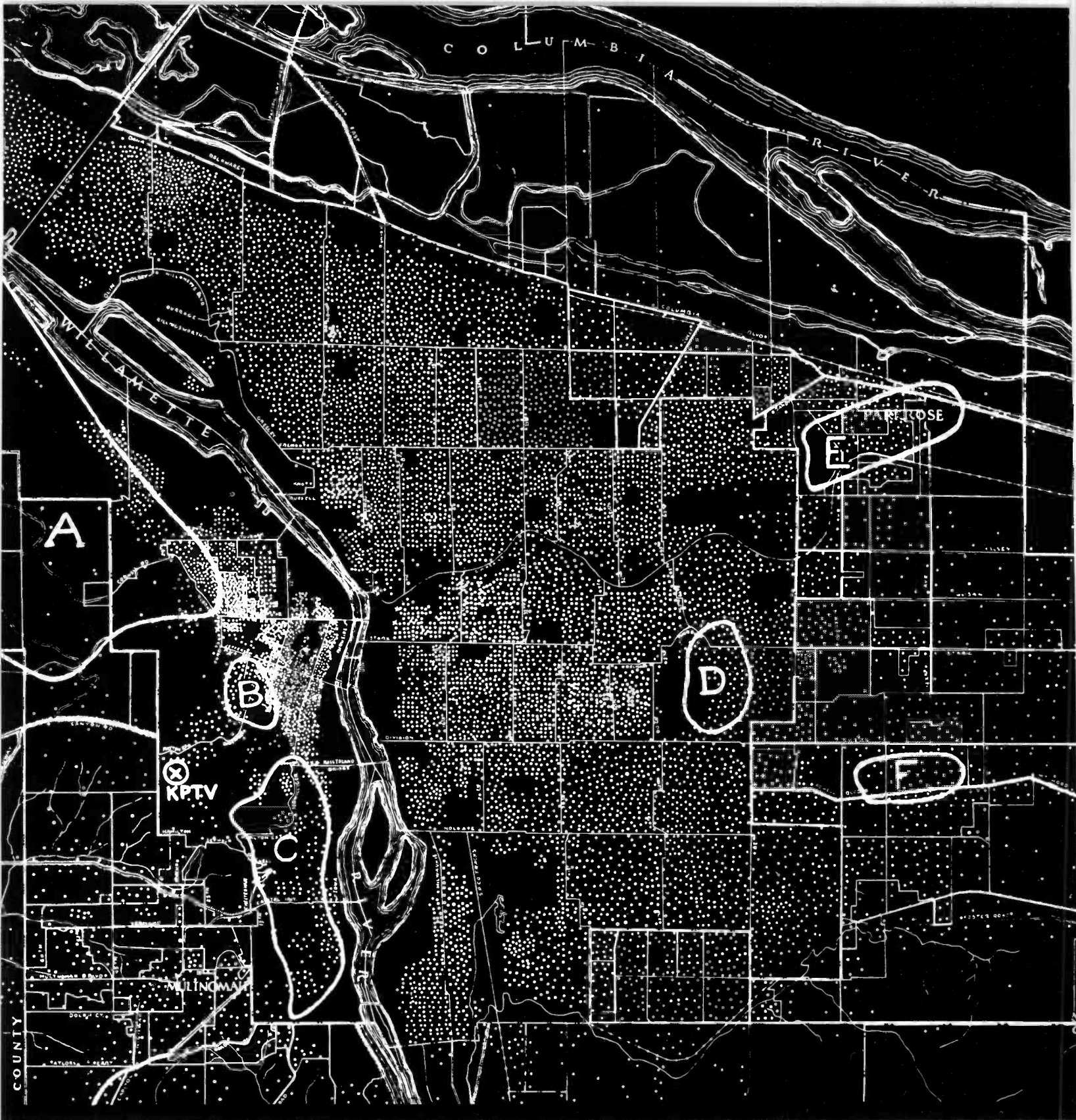
A "population distribution" map of the city of Portland, Oregon. Each dot represents 40 people according to the 1950 census. "A," "B," "C," "D," "E," "F" are areas of poor or no reception and by counting the dots in these regions it was possible to determine the percentage of the population unable to get good reception. With an increase in power of the transmitter and improvements in receivers it is probable that these areas would be substantially reduced in size in the future.
