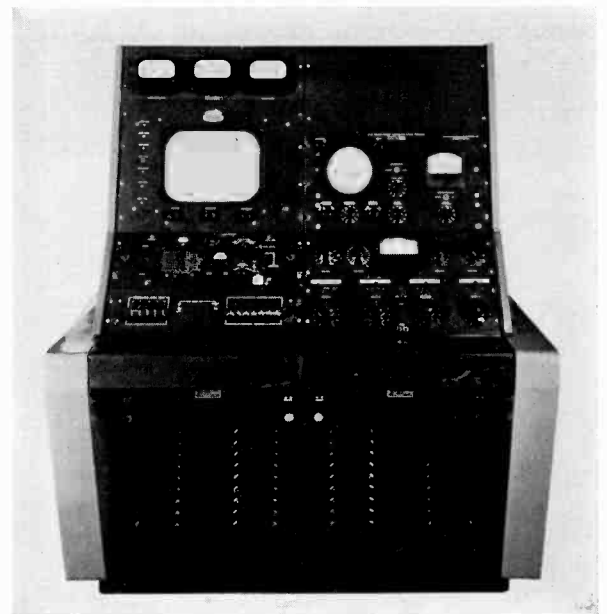
The Dumont control and switcher console.
