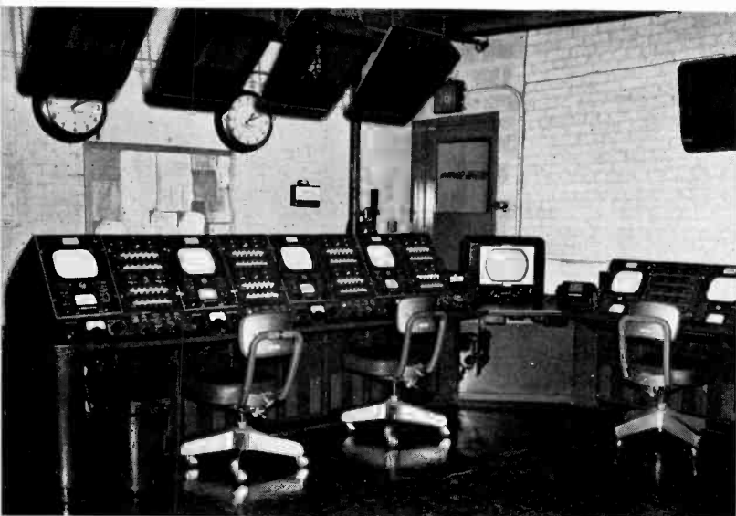
(Left) Another section of the WOR-TV master control room showing video and audio master equipment for centralized operation. (Below) The switch console and transmitter control units which are used in the transmitter room of WJAC-TV in Johnstown, Pennsylvania.
