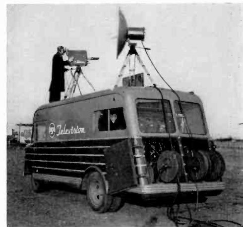
An old mobile unit in operation illustrating a typical field pickup with the camera and microwave transmitter mounted on the roof of the truck. Though their functions differ, the microwave transmitter and receiver are similar in appearance.
