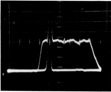
Fig. 14-4. Typical sideband response after adjustment within FCC specifications.
