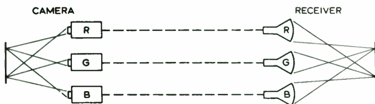
Figure 8.1 Simultaneous 3-wire colour television
