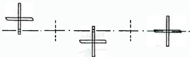
FIG. 49.—This shows the Baird optical lever. The scanned image is thrown onto a ground glass indicated by the vertical dotted line. This is scanned by a second disc and so on. The last disc supplies the up and down motion.
