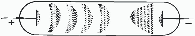
FIG. 33.—When a certain stage of rarefaction is reached in a discharge tube the glow breaks up into striations.
