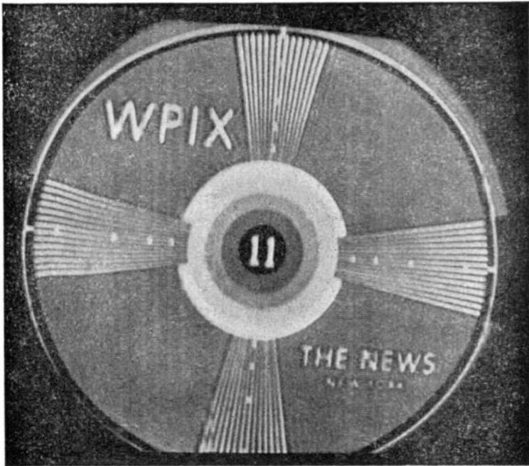
FIG. 16-16. The shadow around the outer edge of the pattern is caused by a deflection yoke which is not as close to the cone of the tube as it will go.
