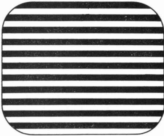
Fig. 16-27. Black and white horizontal bars for checking vertical linearity.
