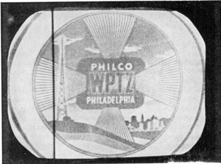
FIG. 16-33. The visual effect of a Barkhausen oscillation.
