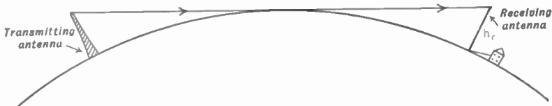
FIG. 2-6. Increase in the line-of-sight distance from the receiving antenna to the transmitter achieved by raising both structures as high as possible.
