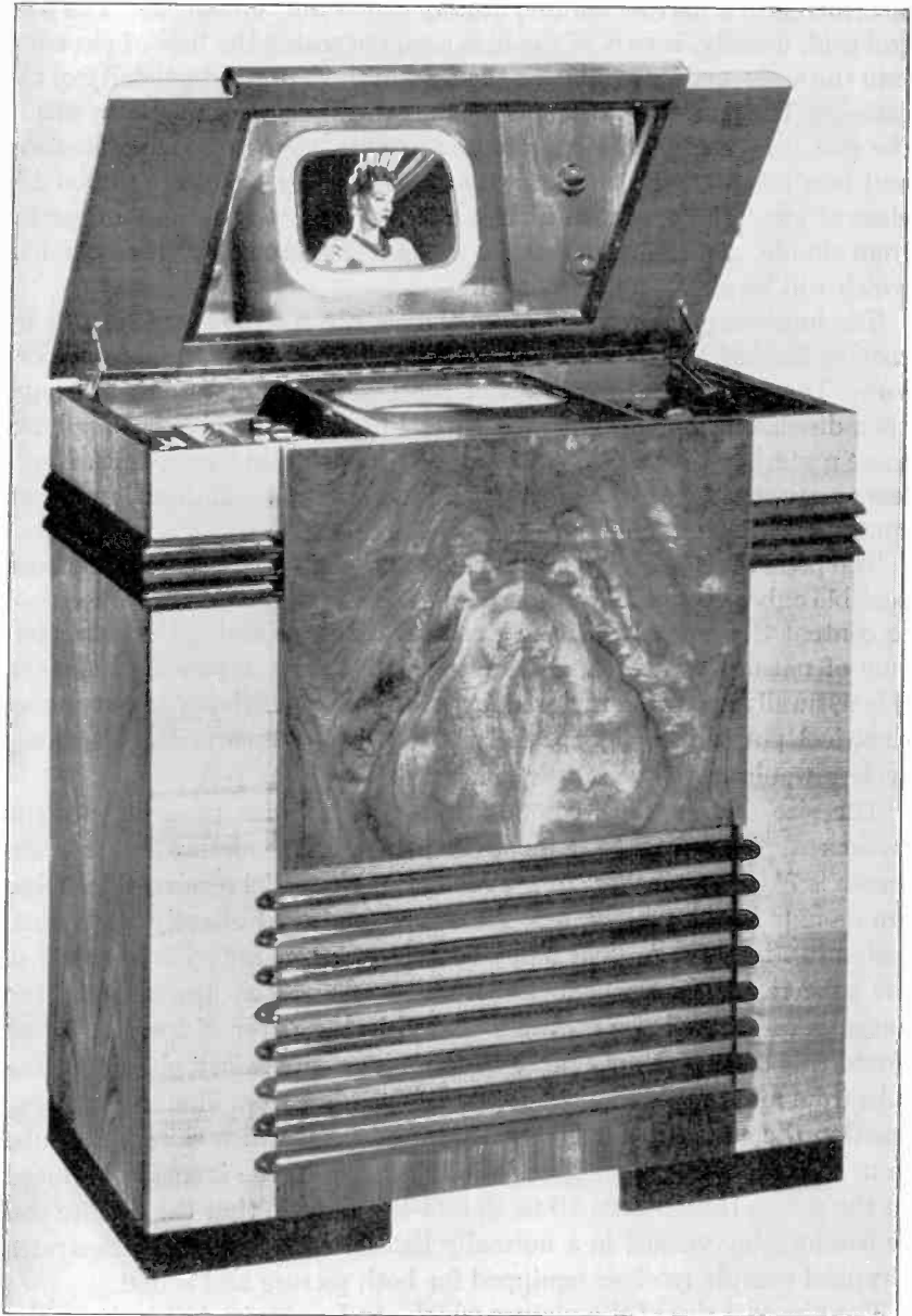
FIG. 9.20.—Console Television Receiver RCA-TRK12.
