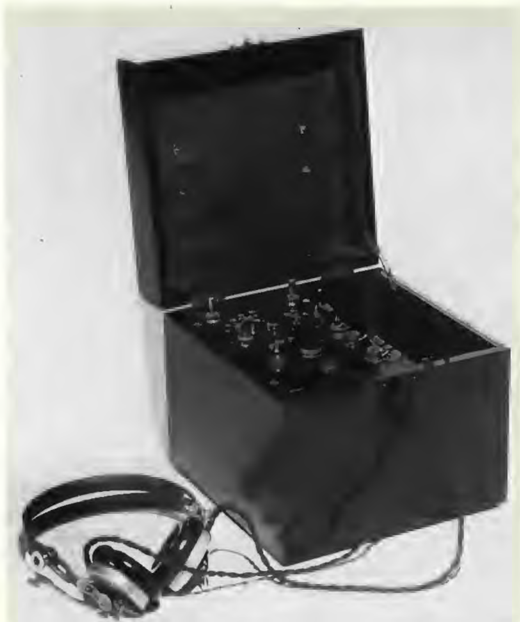
39 Elwell No. 11 crystal set, 1922. Polished ebonite panel with nickel-plated fittings and Tellite crystal, Mahogany cabinet with lid and compartment for headphones.
