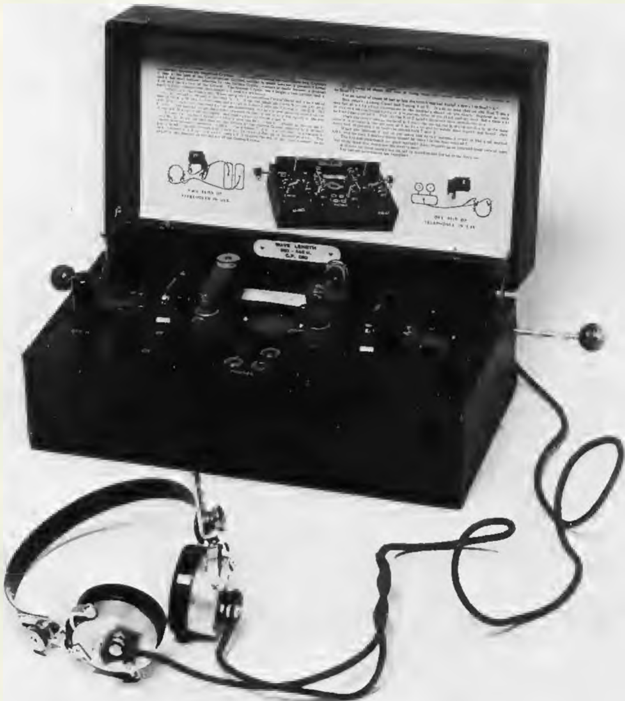
63 Marconi Crystal 'A' crystal set, 1922. Flexine covered case. Wavelength cards can be plugged in behind the detectors to give different wavebands. Shown at the Agricultural Hall Wireless Exhibition, and priced at £9 10s (£9.50).
