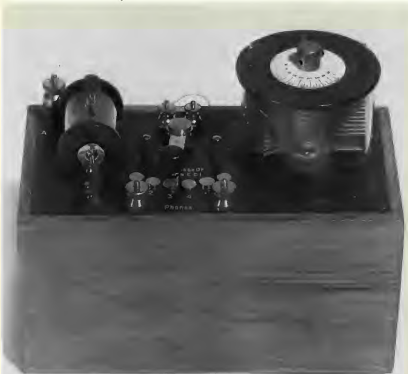
34 Crystal set manufactured by A. W. Gamage Ltd. in 1922. The case is not original.
