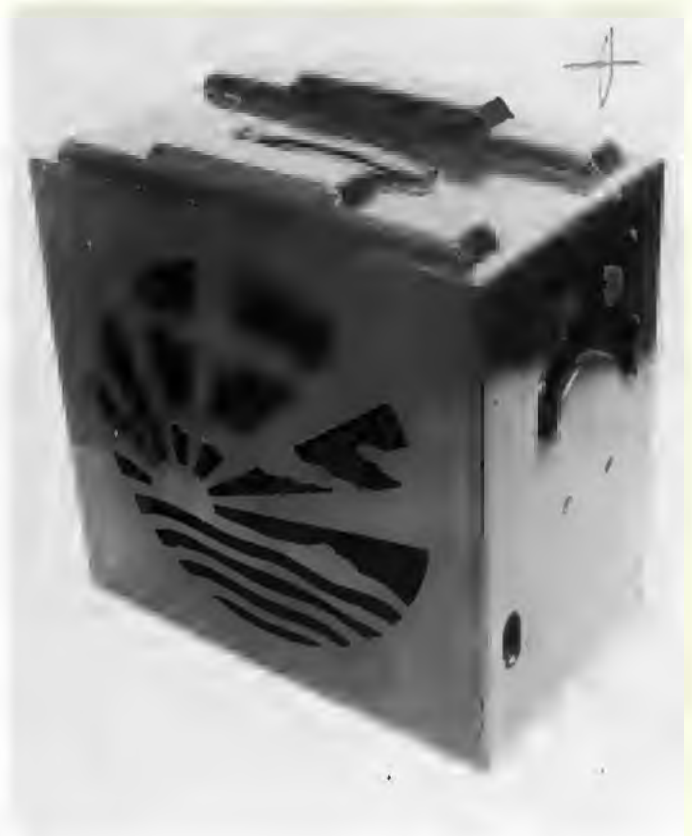
103 Pye Model 'O' Portable, 1932. Built-in frame aerial and moving coil loudspeaker. Cabinet on turntable base.
