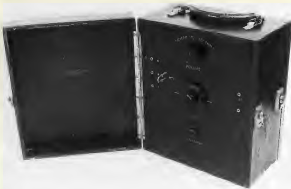
85 The M.P.A. Inclusive Three, a three-valve portable receiver c. 1927. Black Bakelite panel with an oak hinged case opening at the front and back. Variable condenser tuning in conjunction with two Tunewell plug-in coils for all wavelengths between 175 and 840 metres
