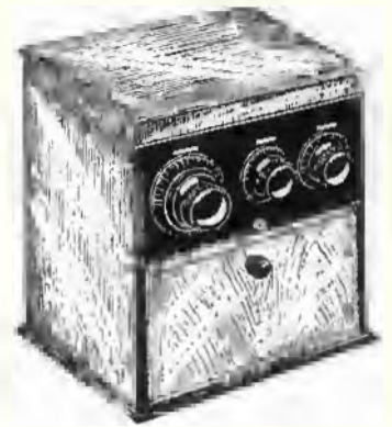
81 Illustration of the first mains-operated set, a receiver by Gambrell Bros. Ltd., 1926.
