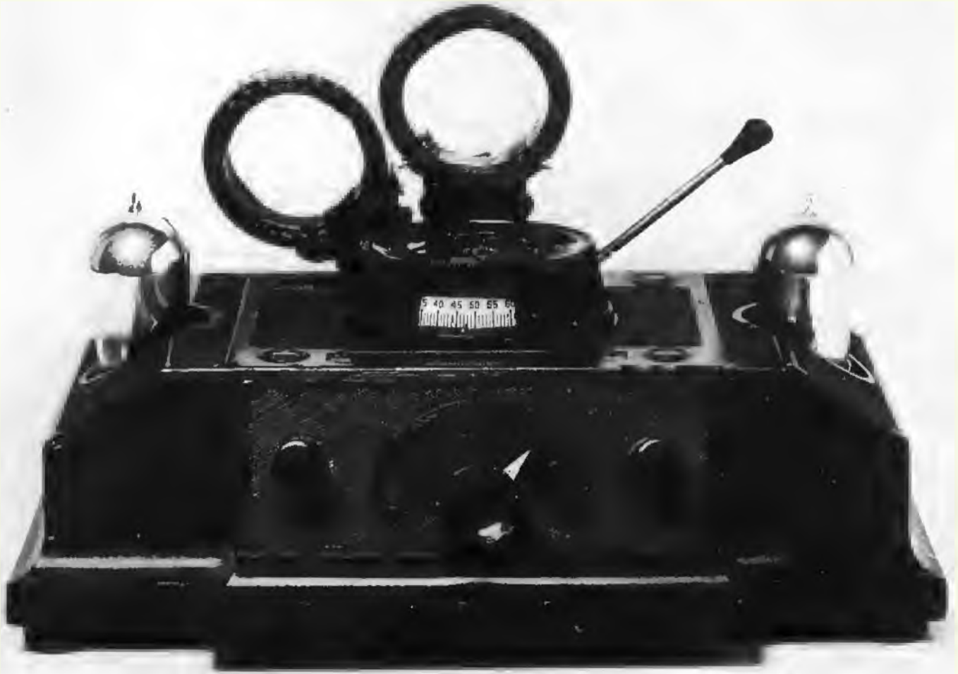
54 Brownie two-valve battery receiver, 1926. It used a loose coupled circuit operating up to 2000 metres and has plug-in coils. Moulded ebonite body. Price: £2 10s (£2.50).
