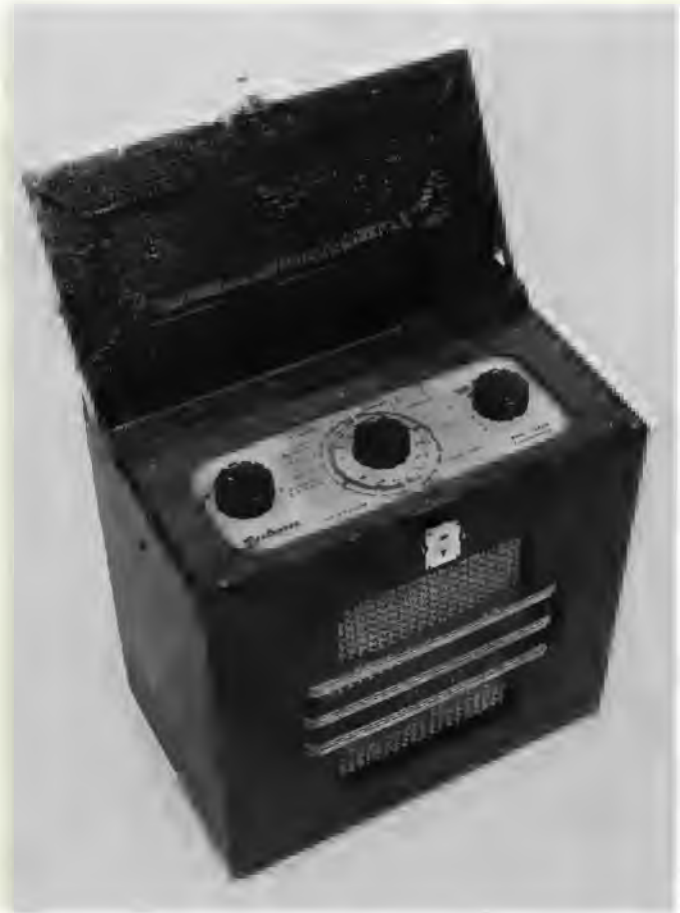
111 Beethoven 'Midget' set of 1934. A mains long and mediumwave receiver, 9½" x 9½" x 6½".
