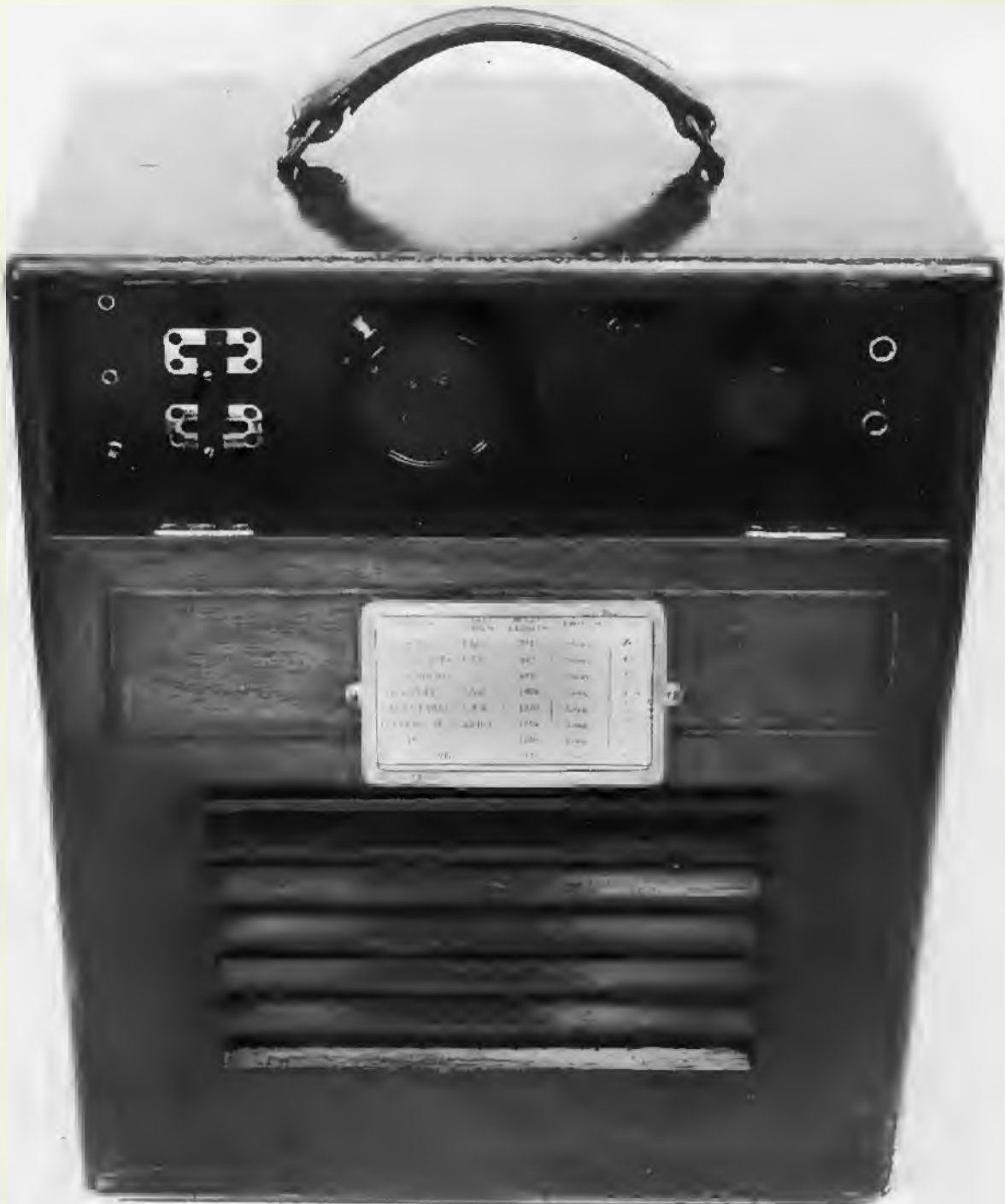
84 Halcyon five-valve portable. 1927. Price: £33 1s (£33.05). Mahogany case with drop-down door revealing the control panel.
