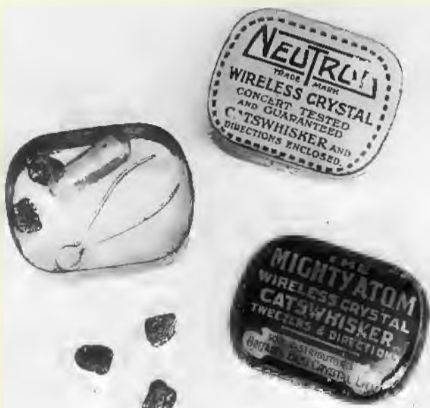
12 Mighty Atom and Neutron wireless crystals and cat's whiskers. In tin boxes complete with tweezers and instructions. Mid-1920s.
