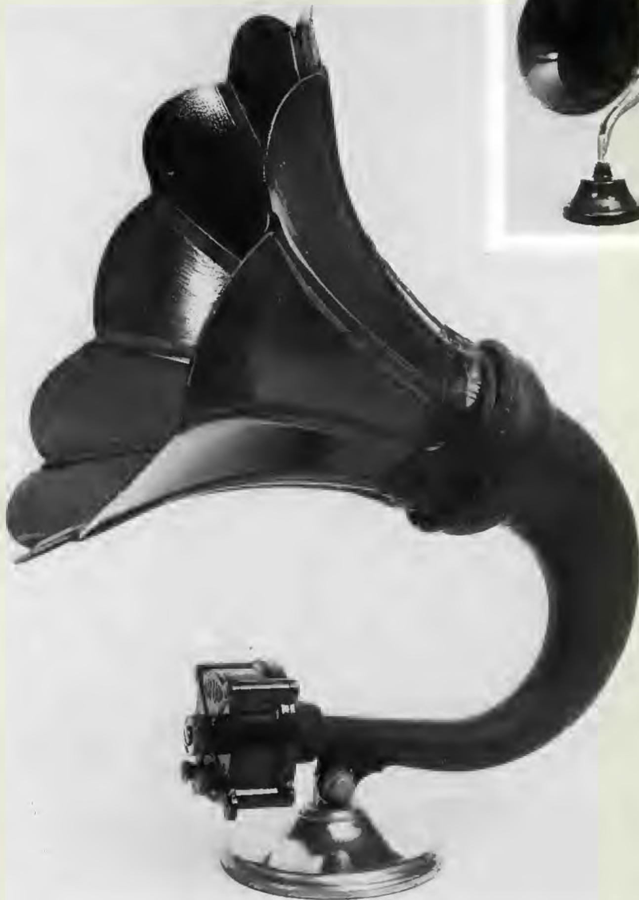
78 Amplion Concert Dragon horn loudspeaker with an oak trumpet, c. 1927. Price: £8 10s (£8.50).
