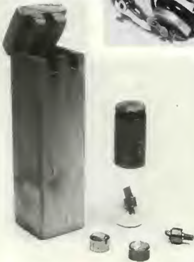
40 Elwell crystals. There are four different kinds of crystals housed in the glass tube, and these can be used in place of the Tellite crystal in the Elwell No. 11 set (ill. 39).
