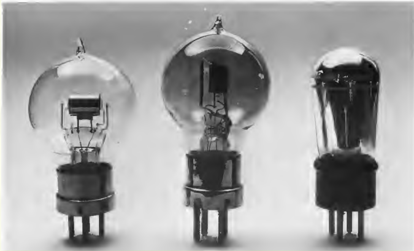
57 Left and Centre: two 'bright emitters' ('R' Type), c. 1923. Right: a Mullard 'Dull Emitter', c. 1925. The silvering which occurred on the inside of valves from the mid-1920s onwards is oxide of magnesium burnt to absorb any traces of gas in the bulb.
