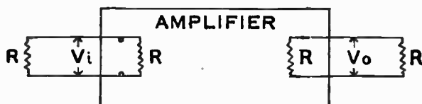
Fig. 1.4 A Symmetrical Amplifier Working between Matched Impedances.
