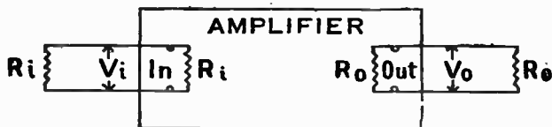
Fig. 1.5 An Unsymmetrical Amplifier Working between Matched Impedances.
