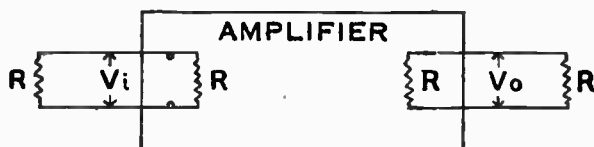
Fig. 1.4 A Symmetrical Amplifier Working between Matched Impedances.
