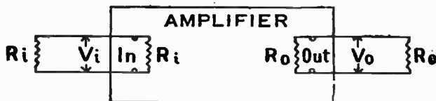
Fig. 1.5 An Unsymmetrical Amplifier Working between Matched Impedances.
