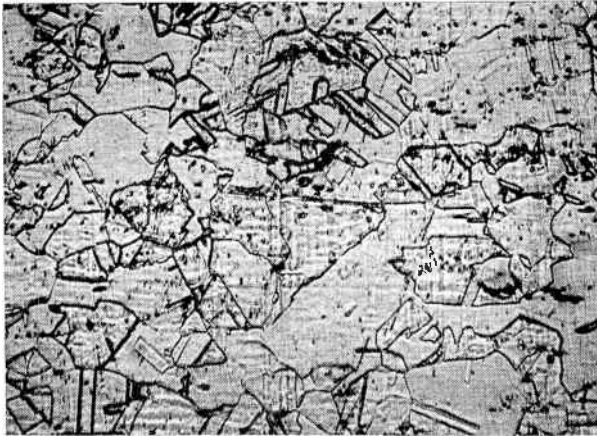
FIG. 1.—A photograph of copper, taken by microscopic means. This is called a photomicrograph and shows the grain or crystal structure of the copper ( Courtesy of Profs. S. H. Graf and C. E. Thomas, Oregon State College ).
