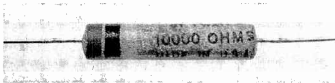
FIG. 35.—Photograph of a resistor of the “composition” instead of wire-wound type. This resistor will only dissipate one watt. They are made in values of from a few ohms to millions of ohms.
