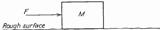
FIG. 39.—Work is done when the force F moves the mass M along the rough surface.
