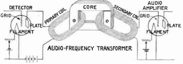
Transformer Construction: The Electric and Magnetic Links
