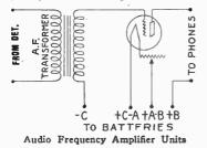
FREQUENCY AUDIO AMPLIFIER UNIT: The wiring of the audio amplifier, as shown in the Circuit Unit Diagram, is subject to but little variation. Practically the only modifications commonly seen are in use or non-use of the "C" battery, unless the circuit is "reflexed," as described below, or unless the "Push-Pull' principle is utilized. Audio Frequency amplification is discussed at greater length in a succeeding chapter, as is also "Push-Pull" amplification.
