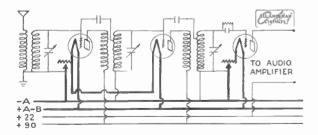
The Neutrodyne has been popular in many quarters on account of its freedom from oscillation (which however depends on exact neutralization for the tubes being used) and on account of its dependability when properly made. It is doubtful, however, whether a Neutrodyne will equal even in these respects the radio frequency hook-up shown on page 46. In distance range, the latter is certainly far superior, particularly when using the loop antenna, for which the Neutrodyne is not very well adapted.
