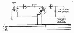
This is one of the "old original" regenerative circuits. The variometer in the plate circuit enables it to be tuned to the proper relation to the grid circuit so that regeneration will take place. The second variometer, in the grid circuit, tunes this circuit to the received signal. Selectivity is fairly good, as a rule. This circuit can be used with a loop antenna for local stations. CHAPTER VIII All-American "OK" Circuits
