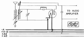
This circuit is quite popular, and splendid results can be obtained with it. Due to the twocircuit or inductive coupling, selectivity is quite high, and with the proper number of turns on the tickler, a very smooth control of regeneration can be secured. As in other regenerative circuits, it is important to have a by-pass condenser across the detector output, and using a larger condenser will increase the amount of feed-back.
