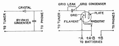
Detector Units: Crystal and Vacuum Tube Types
