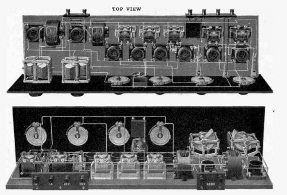
An Eight Tube Thirty Kilocycle Super-Heterodyne Receiver of Advanced Design, Utilizing the All-American Radio Frequency Coupler, 10,000 Meter Transformer, Long Wave Transformers, Standard Audio Transformers, and Tube Sockets. A Wiring Diagram of this Set Will be Found on Page 47
