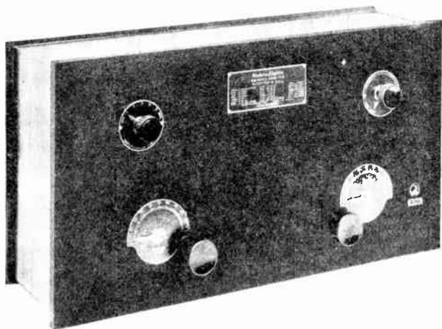
FIG. 248a. Western Electric 4-D Radio Receiver (Double-Detection).
