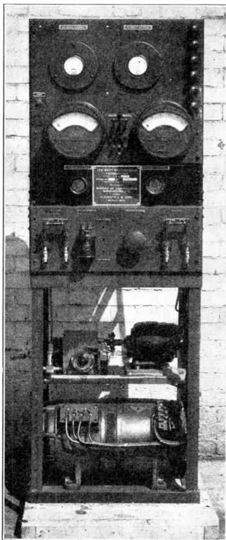
FIG. 249a. U. S. Bureau of Lighthouse 100-Watt Radio Beacon Transmitter with Automatic Signaling Device.
