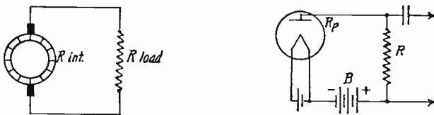
FIG. 87. The Output Rule—Showing that when Load Resistance is Equal to Internal Resistance Maximum Output is Obtained.
