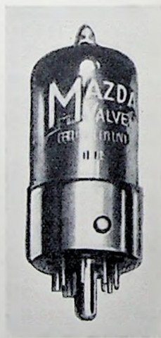
FIG. 6.7H. THE 6F13; AN EXAMPLE OF THE NEW MINIATURE U.H.F. SIGNAL AMPLIFIER PENTODES (Courtesy of Edison Swan Electric Co., Ltd.)
