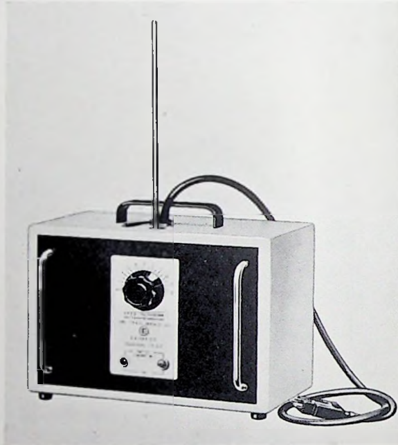
FIG. 10.3B. THE EKCO PATTERN GENERATOR
