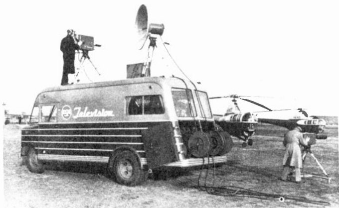
Figure-107. (A) Floor plan and (B) exterior appearance of mobile television unit. (courtesy RCA)
