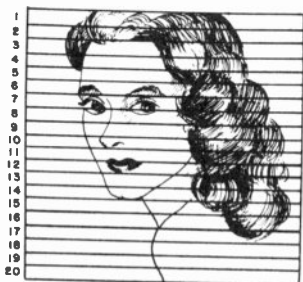
Figure 9. How linear scanning is accomplished.
