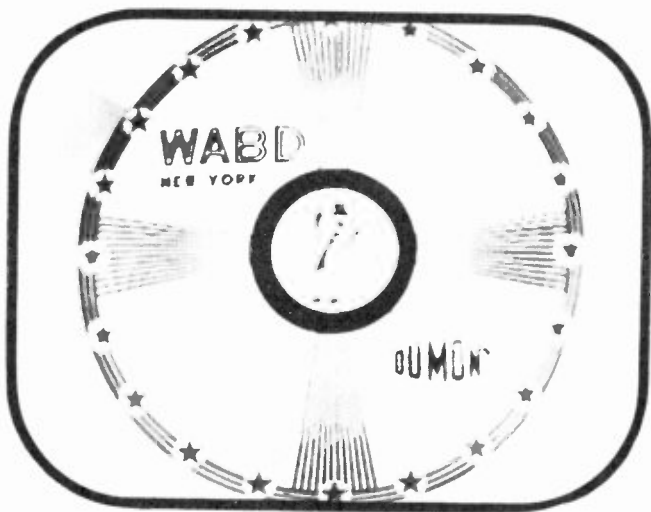
Figure 68B Test pattern with poor resolution, as it appears on screen of picture tube.
