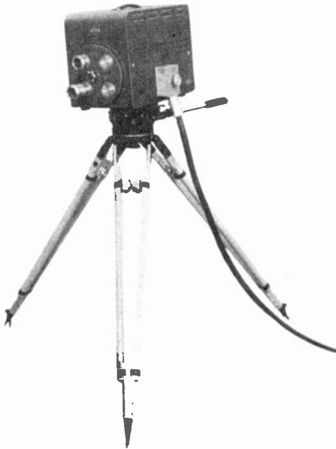
Figure 72. Pickup head mounted on tripod for remote pickup use. (courtesy Raytheon)
