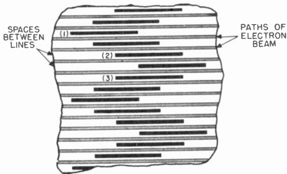
Figure 66. Magnified portion of the mosaic showing scanning lines and pattern of horizontal black lines projected on the mosaic.
