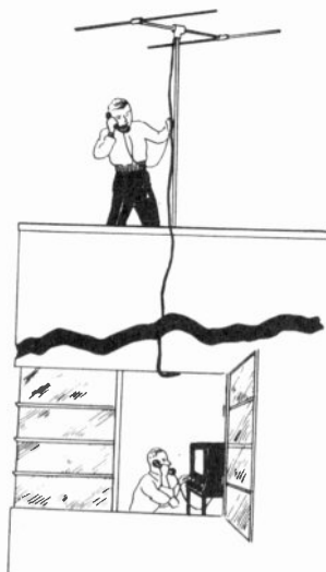
Figure 5. Sound-powered phones connected through transmission line help in locating antenna.
