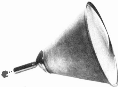
Figure 130. Picture tube with metal funnel.
