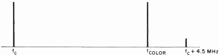
Fig. 4-4 Placing the color carrier further from the video carrier tends to reduce interference effects.
