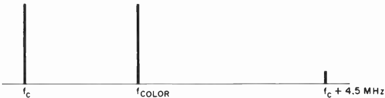
Fig. 4-3 Locating the color carrier adjacent to the video carrier will produce strong interference patterns.
