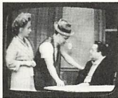
INCORRECT VERTICAL SIZE OF PICTURE; SOUND OK. REMEDY: K
