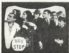
BOWED SHAPE OR "PINCUSHION" AT TOP (OR BOTTOM); SOUND OK. REMEDY: I
