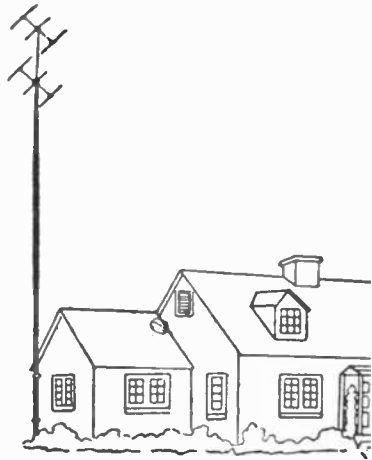
Fig. 7. A typical fringe-area antenna installation.
