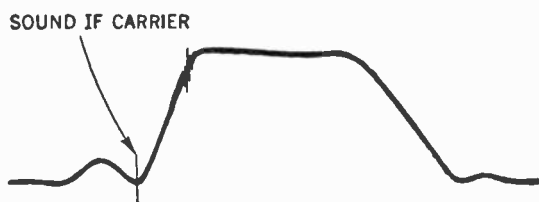
Fig. 10. Trace of video IF response with sound carrier frequency marked.
