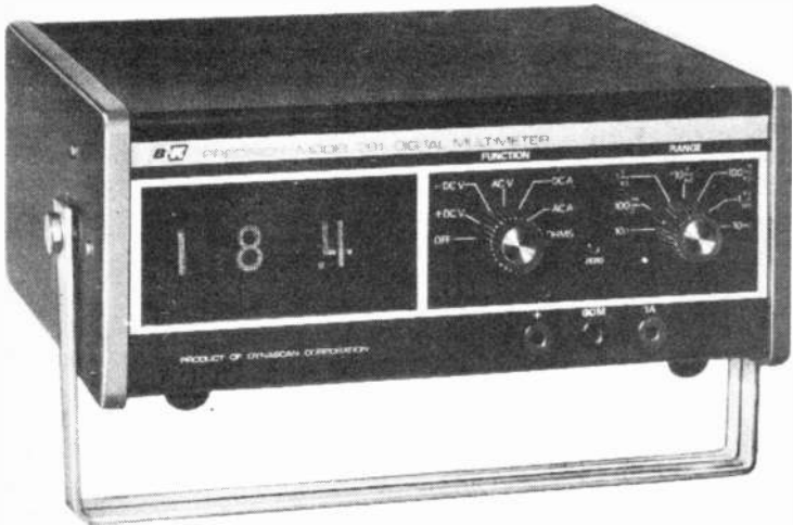
Courtesy B&K Precision, Div. of Dynascan Corp. Fig. 10. A typical digital multimeter.
