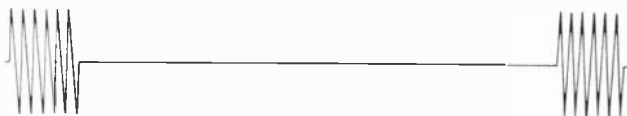
Fig. 16. The output from Q6 in Fig. 15 is a train of pulsed bursts.
