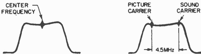
Fig. 12. Trace of typical RF response.
