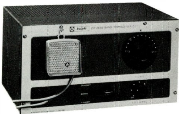
Fig. 1212. Front-view of a Citizens-band transceiver. Minimum number of controls gives this unit a clean look, makes it easy to operate. (Allied Radio Corp.)
