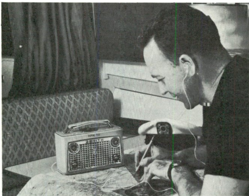
Fig. 1002. Two-band transistor portable covers the standard AM broadcast band and the radio-beacon band. (Zenith Radio Corp.)
