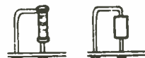
Fig. 1205. Schematics that come with imported receivers include more information than we are used to seeing. Here component polarity is indicated. In compact units component size and height are important. (Sony)
