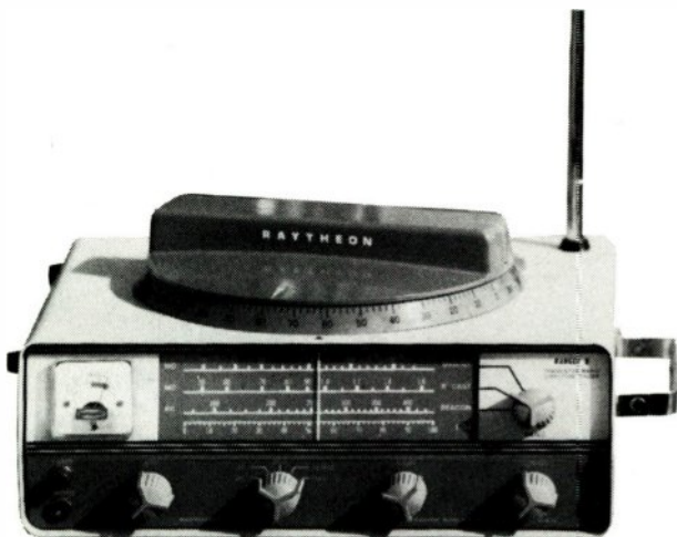
Fig. 1007. This portable radio direction finder receives signals from long-range Consolan stations and standard broadcast bands as well as regular marine beacons. Sense antenna, right rear, differentiates between correct bearings and reciprocal bearings. Six standard flashlight batteries power the receiver. A dual purpose meter indicates battery strength and provides visual null reading for accurate bearings. (Raytheon Co.)
