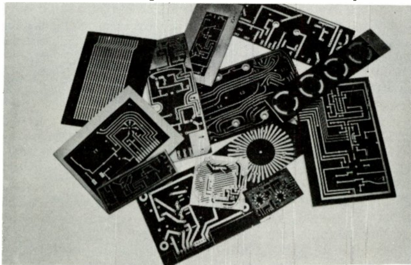
Fig. 212. Printed-circuit boards come in a large variety of sizes and shapes. They are used in AM, FM and TV receivers, test equipment and components like rotary switches, commutators, loop antennas, meter coils and motor armatures. (Keil Products)
