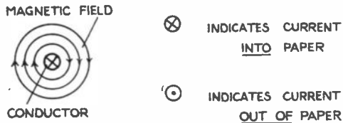
FIG. 7.1. MAGNETIC FIELD ROUND A CONDUCTOR
