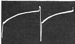
6BL7GT (V15) Vertical Oscillator Control Grid (Pin 1) 600 Volts P/P Vertical
