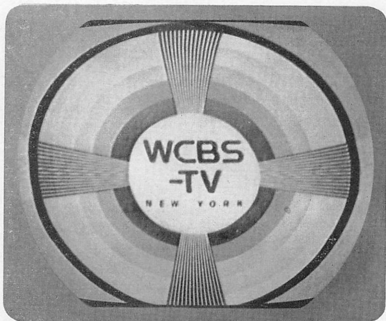
FIG. 3-50 WAVY LINES ACROSS PART OF PICTURE • SOUND NORMAL •
