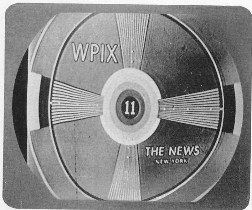
FIG. 3-35 HORIZONTAL NON-LINEARITY • SOUND NORMAL •
