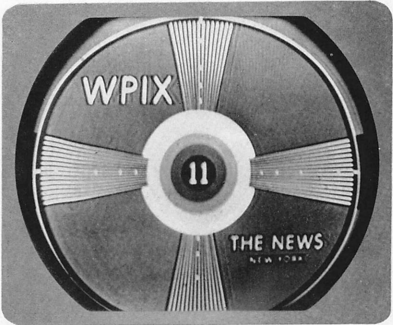
FIG. 3-17 SHADOW AROUND PICTURE • SOUND NORMAL •
