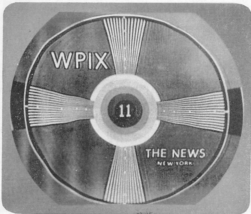
FIG. 3-45 PICTURE HAS "WRINKLED" APPEARANCE • SOUND NORMAL •
