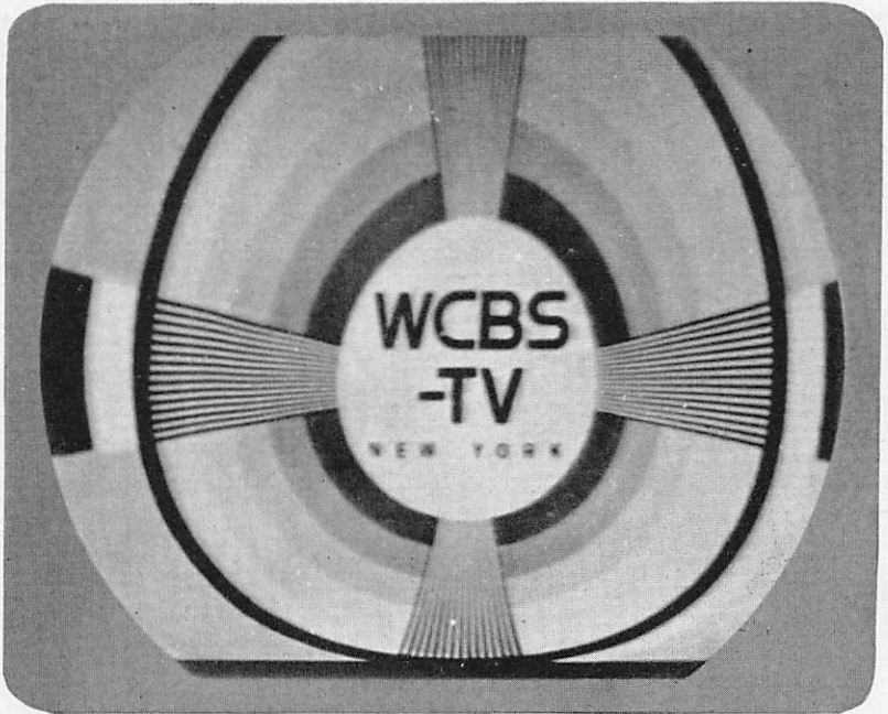
FIG. 3-34 VERTICAL NON-LINEARITY • SOUND NORMAL •
